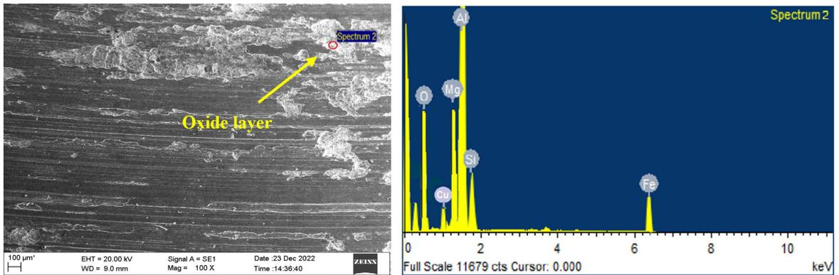
Figure 16. EDAX results of C2 composite at applied load of 40 N.
