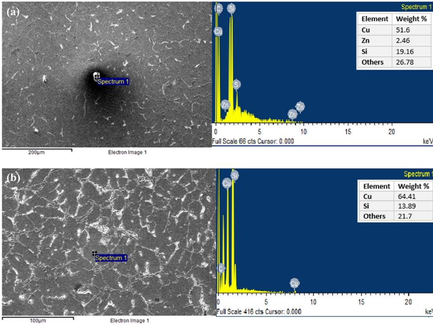
Figure 7. EDAX report showing the presence of (a) Cu coated Zn in C1 composite and (b) Cu in C2 composite.
