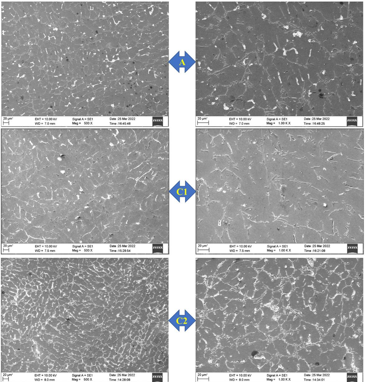
Figure 5. SEM images of as-cast matrix A, C1 and C2 composite.
