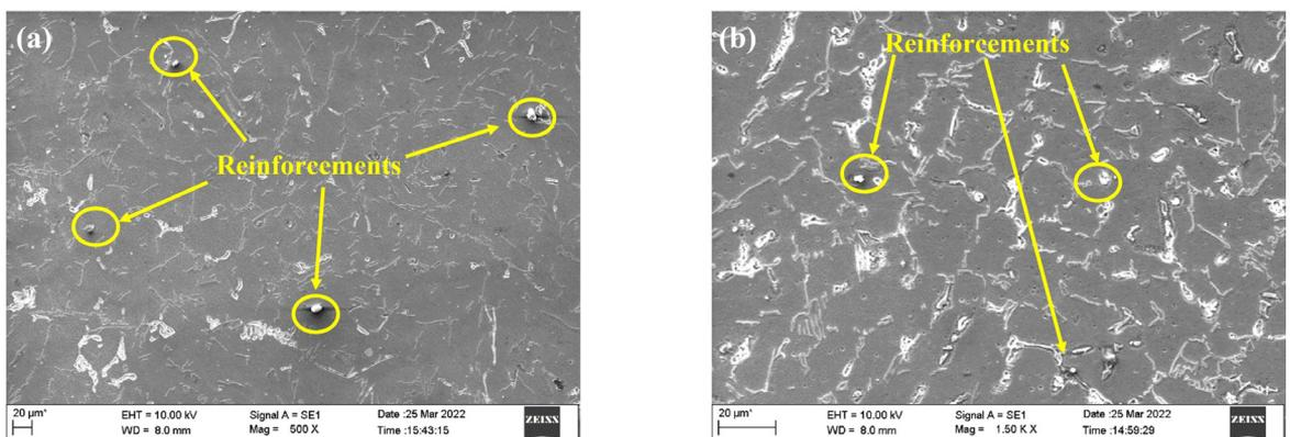
Figure 6. Reinforcement distribution of (a) C1 and (b) C2 composites.
