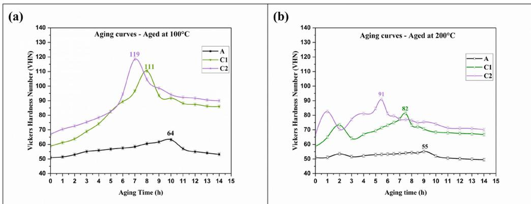
Figure 9. Aging curve of composites compared with matrix alloy A aged at (a) 100°C (b) 200°C.
