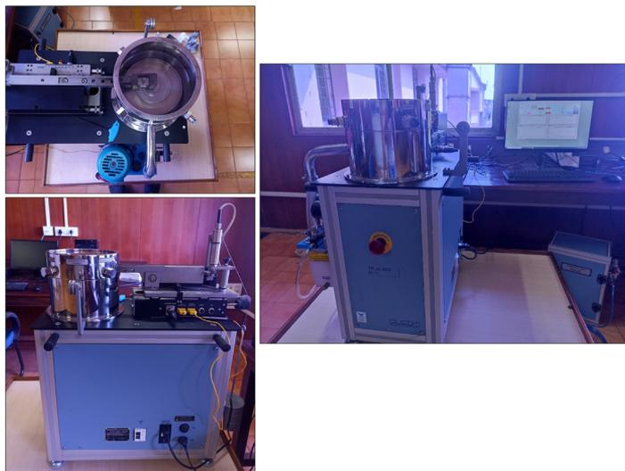
Figure 3. Pin-On-Disc tribometer.
