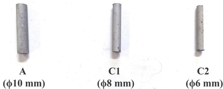
Figure 2. As-cast pin specimens used for wear test.
