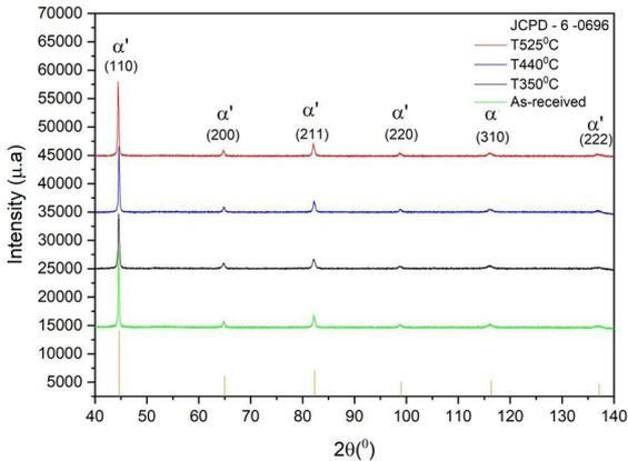
Figure 7. API 5CT P110 steel diffractogram.
