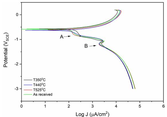
**Figure 3.** Potentiodynamic polarization curves in NaCl (0.42M),  $T=25^\circ\text{C}$ .
