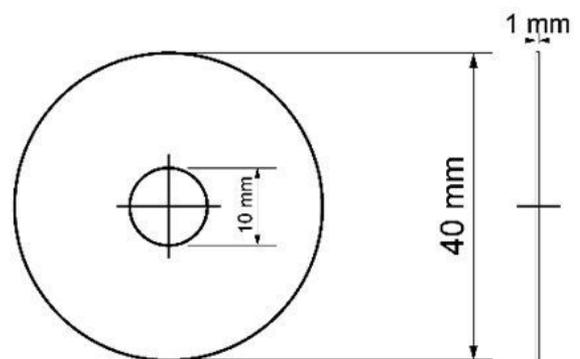
Figure 1. Schematic of samples used in electrochemical tests<sup>27</sup>.
