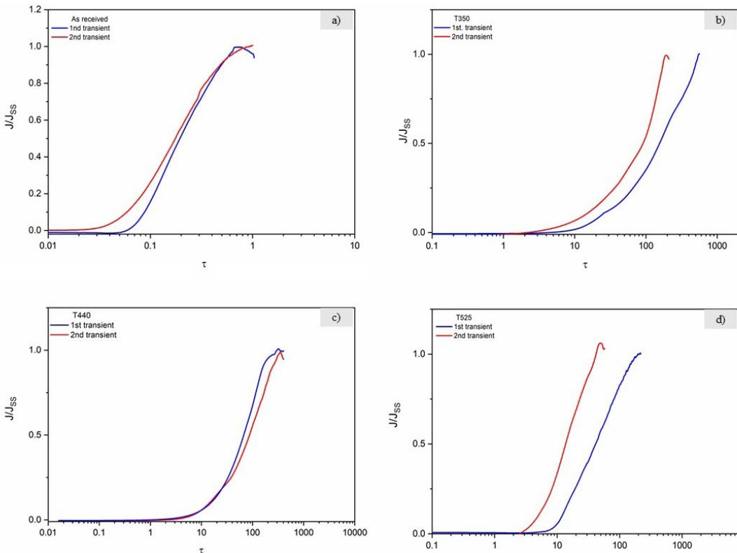
Figure 4. Normalized permeation curves (a) as-received; (b) T350; (c) T440; (d) T525.
