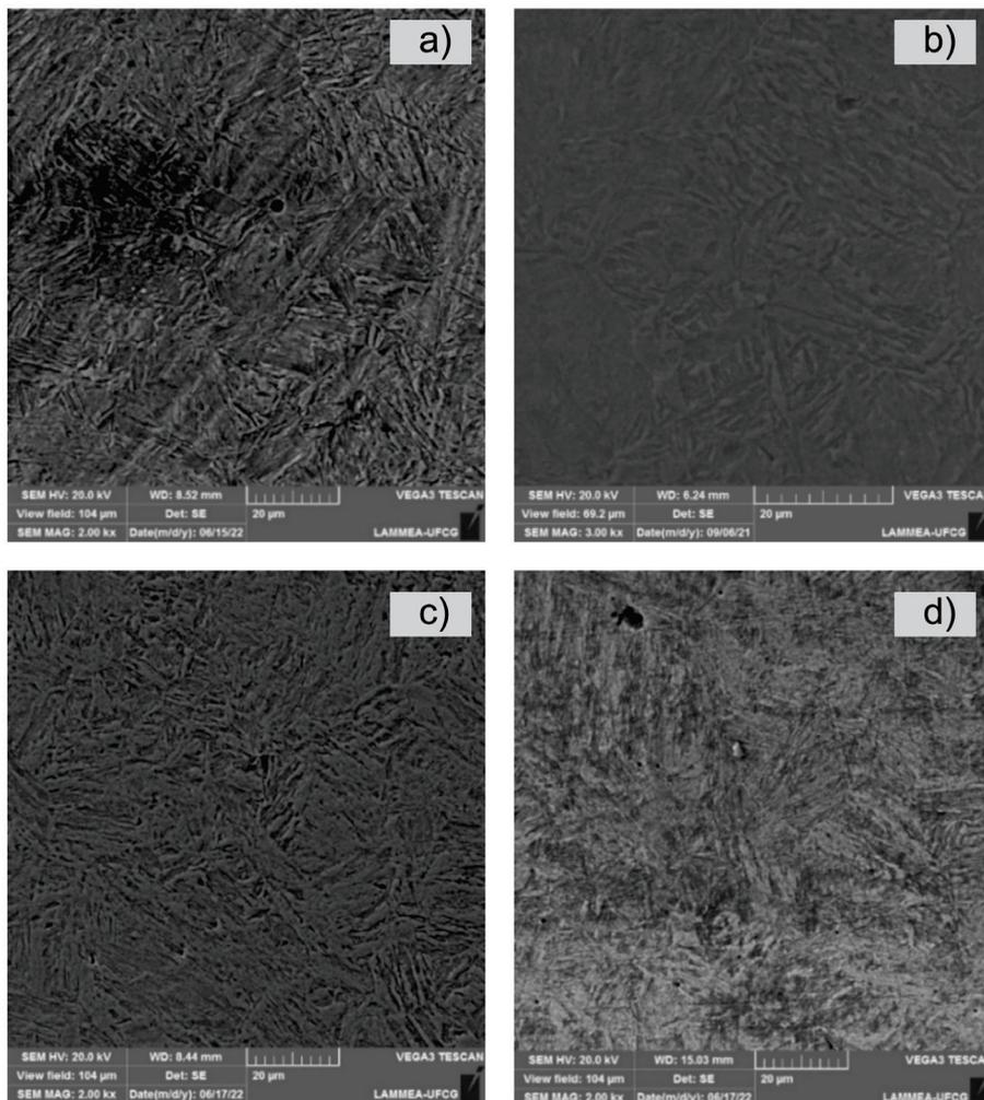
**Figure 5.** Material microstructure. (a) As-received; (b) T525; (c) T440; (d) T350.
