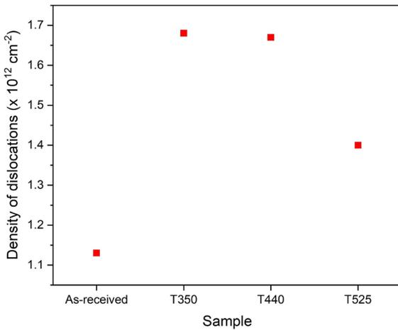
Figure 8. Density of dislocations as a function of tempering temperature.
