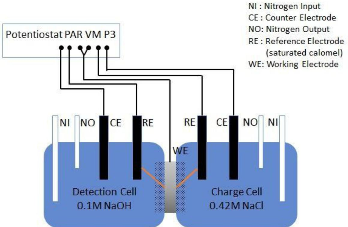
Figure 2. Schematic of double-cell used in electrochemical tests.
