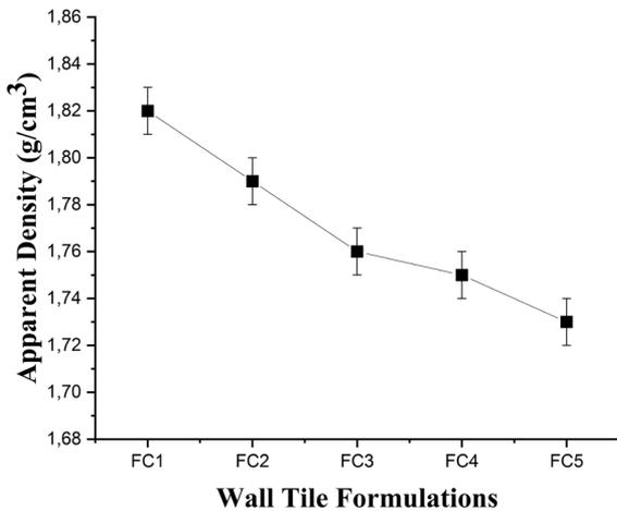
Figure 7. Apparent density of the red wall tile pieces.
