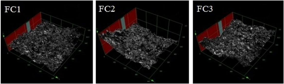
Figure 5. 3D confocal images of the fired red wall tile pieces (Magnification: 430x).
