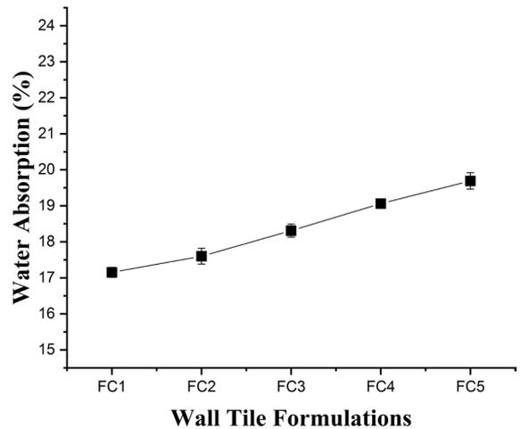
Figure 8. Water absorption of the red wall tile pieces.
