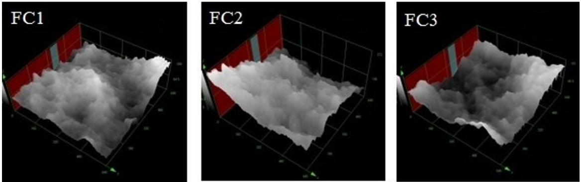
Figure 6. 3D confocal images with noise filter of the fired red wall tile pieces (Magnification: 430x).
