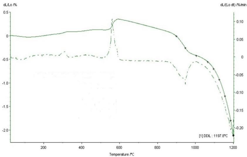
Figure 4. Dilatometric analysis for the FC3 formulation.
