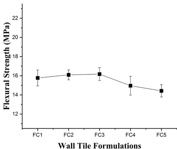
Figure 9. Flexural strength of the red wall tile pieces.
