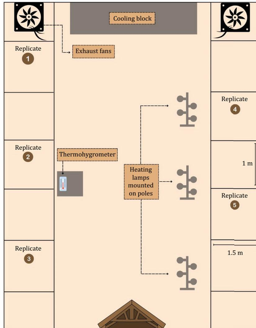
**Figure 1** - Climatic chamber used with the necessary equipment to control and measure temperature.
