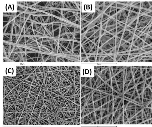
**Figure 1** Morphology of electrospun (A) PLLA, (B) PLLA-collagen (C) Gelatin (D) PLLA-Gelatin scaffolds (Scale bar = 2  $\mu$ m).
