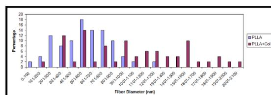
**Figure 2** Fiber diameter range of electrospun nanofibers prepared from PLLA and PLLA-Collagen
