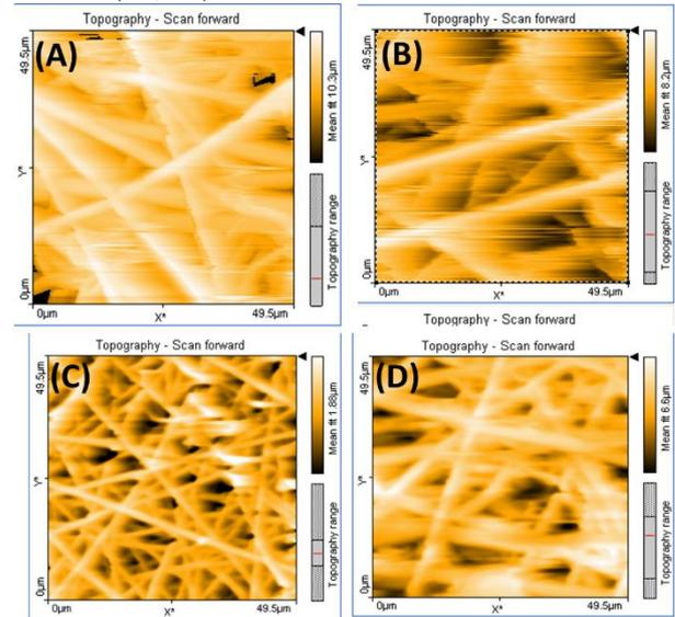
**Figure 4** Mean fit AFM images of electrospun nanofibers of (A) Pure PLLA (B) PLLA-Collagen(C) Pure Gelatin and (D) PLLA-Gelatin
