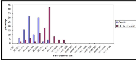
**Figure 3** Fiber diameter range of electrospun nanofibers prepared from Gelatin and PLLA + Gelatin
