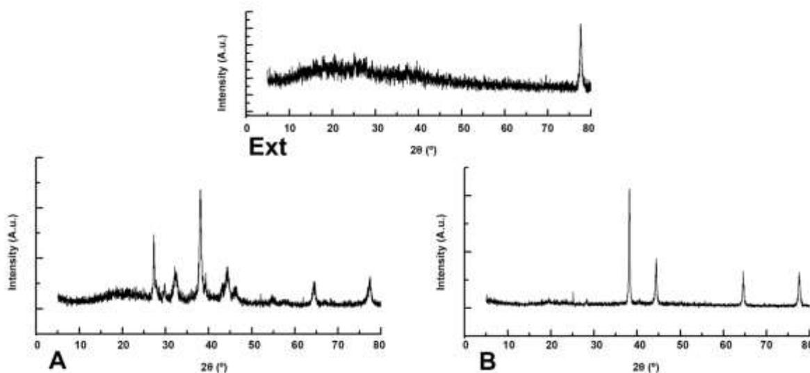
**Figure 4.** X-ray diffraction of aqueous extract (Ext) and nanoparticles obtained from silver (A) and gold (B).
