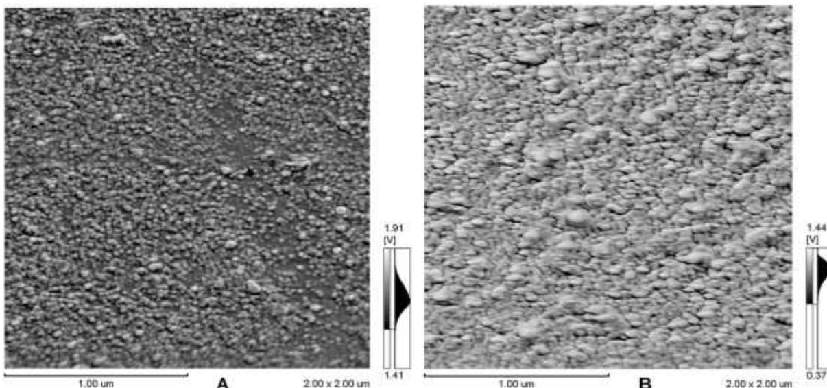
**Figure 2.** Images of nanoparticles obtained by TEM technique for silver (A) and gold (B) nanoparticles.
