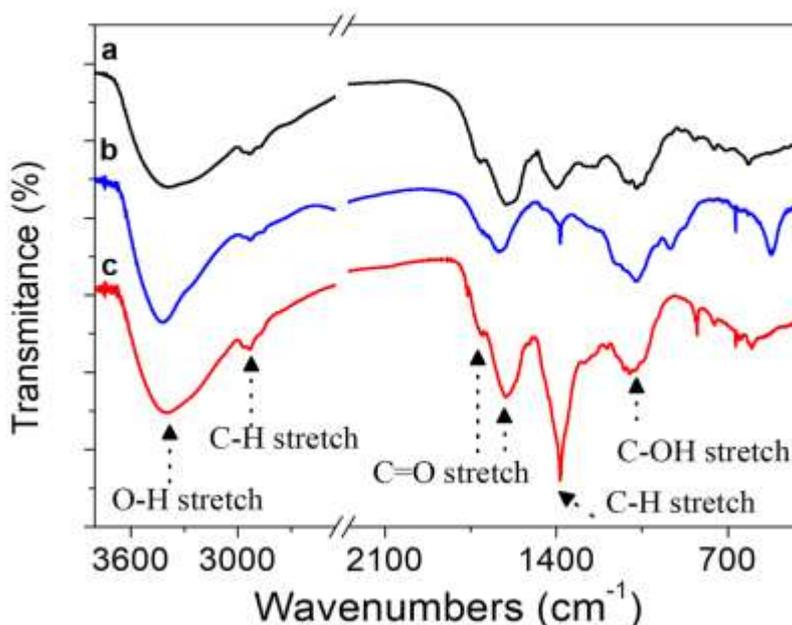
**Figure 5.** FTIR spectrum of aqueous extract of *Lavandula dentata* (a) and obtained nanoparticles with silver (b) and gold (c).
