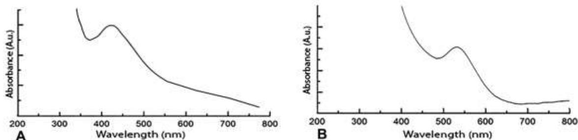
**Figure 1.** UV-Vis spectra of nanoparticles obtained with silver (A) and gold (B).
