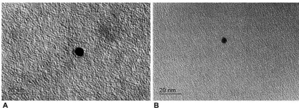
**Figure 3.** Images of nanoparticles obtained by TEM technique for silver (A) and gold (B) nanoparticles.
