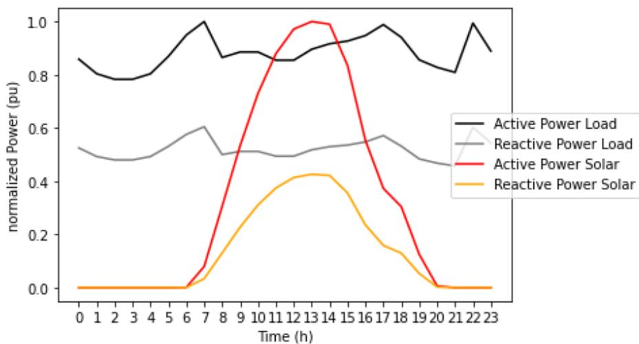
**Figure 2.** Load and Solar Profiles per unit.
