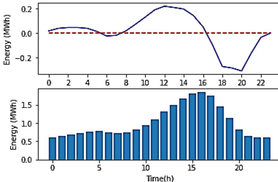
**Figure 8.** BESS power and energy behavior at bus 9 when scenario 4 is considered.
