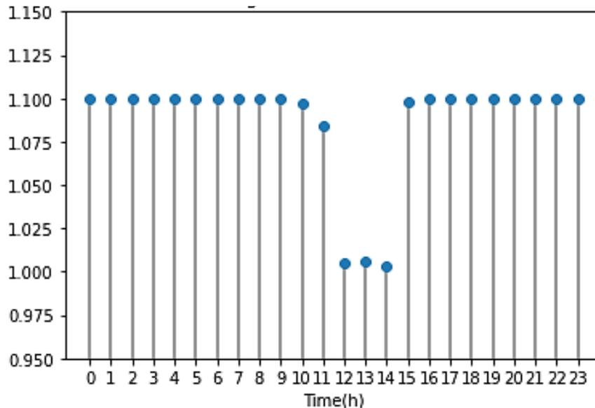
**Figure 7.** Voltage Regulator TAP positions when scenario 4 is considered.
