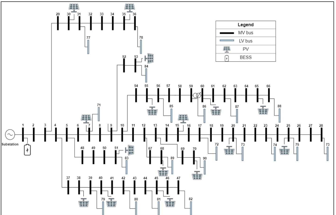
**Figure 1.** 90 Buses Test Circuit. Adapted from [6].
