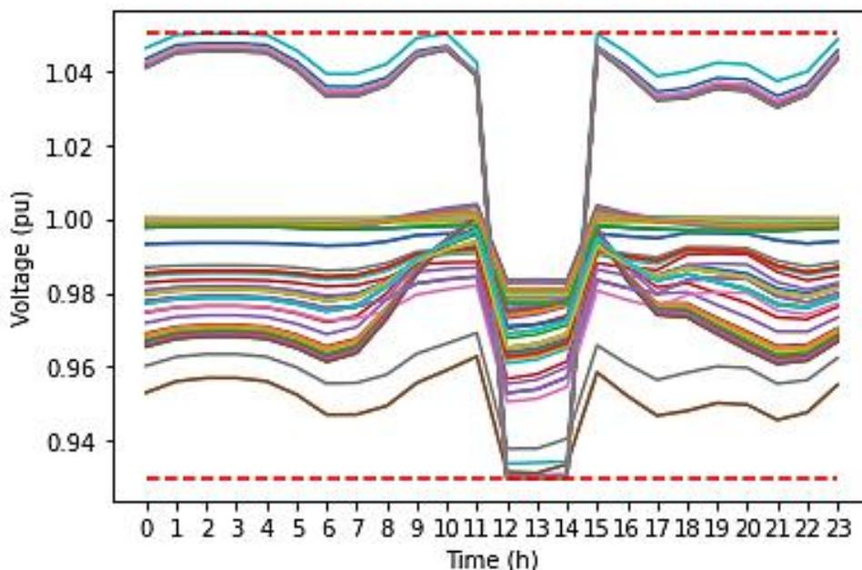
**Figure 6.** Voltage in all circuit buses when scenario 4 is considered.
