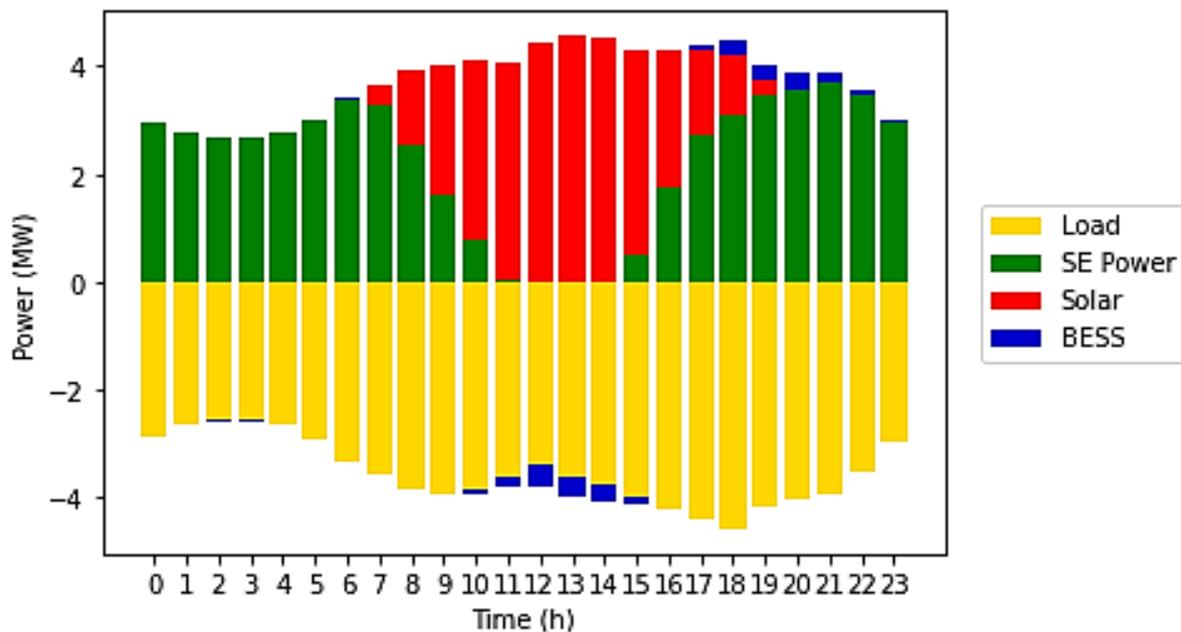
**Figure 4.** Active power balance at the substation bus at scenario 4.
