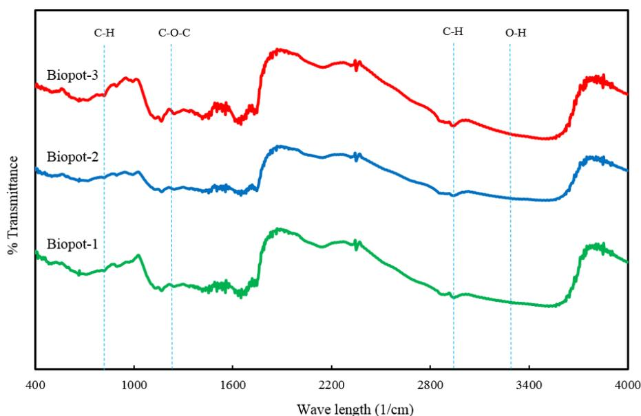
**Figure 7.** FTIR Spectra of the examined biopots.
