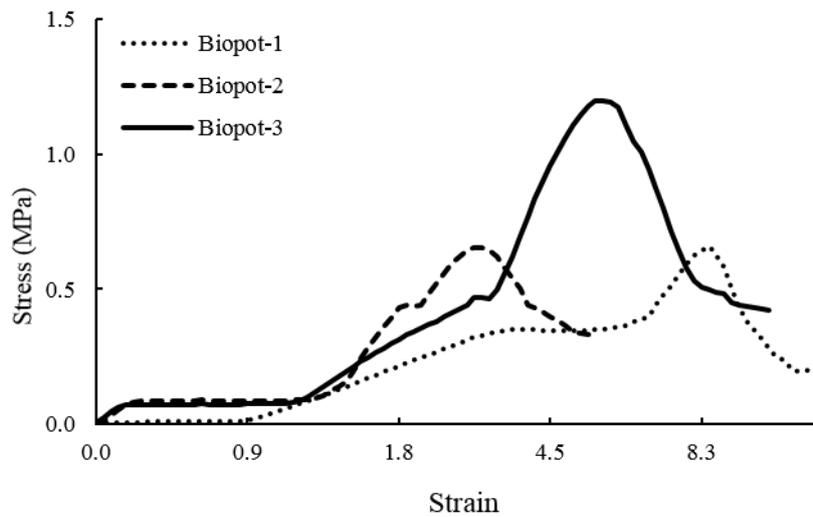
**Figure 6.** Curve of stress-strain of the examined biopots.
