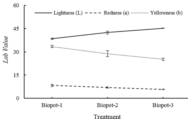
**Figure 2.** Colorimetric value of the tested biopots.
