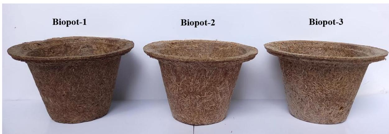
**Figure 1.** Physical appearance of the produced biopots - Biopot-1 (5% sodium alginate); Biopot-2 (10% sodium alginate); Biopot-3 (15% sodium alginate).
