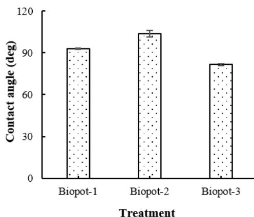
**Figure 3.** Contact angle of the examined biopots.
