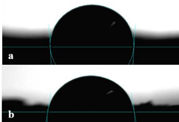
**Figure 4.** Contact angle of Biopot-3 with hydrophobic angle of  $<90^\circ$  (a) and Biopot-2 with hydrophilic angle of  $>90^\circ$  (b).
