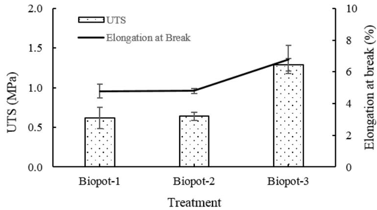
**Figure 5.** Ultimate tensile strength (UTS) and elongation at break of the examined biopots.
