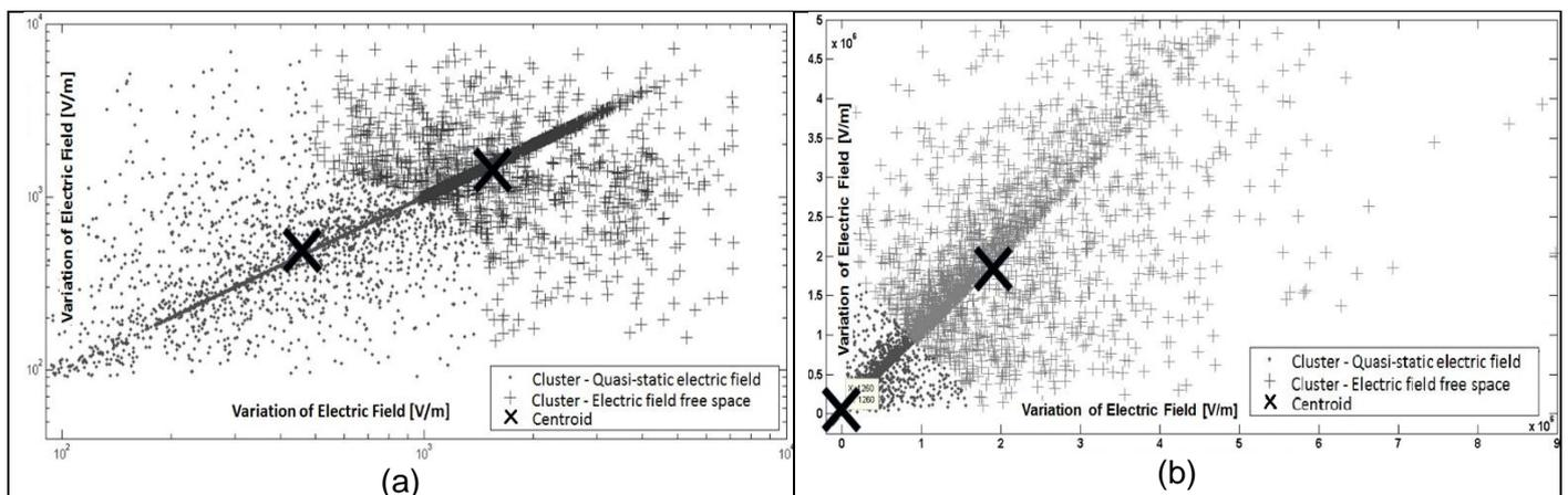
**Figure 4.** (a) Clustering of the measured and calculated electric field values for the EHF range; (b) Clustering of the measured and calculated electric field values for the VLF range.
