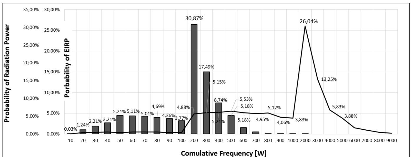
**Figure 7.** Cumulative frequency of EIRP values (line) and irradiated power (bar), both in [Watt], and the respective probability values.
