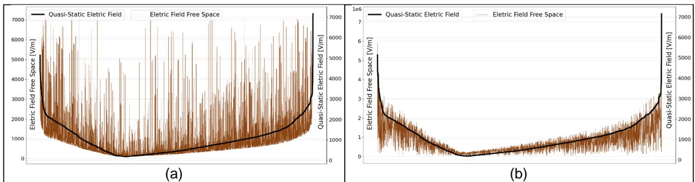
**Figure 5.** (a) Absolute values of the quasi-static and free space electric fields, considering waves in the EHF range. (b) Absolute values of the quasi-static and free space electric fields, considering waves in the VLF range.
