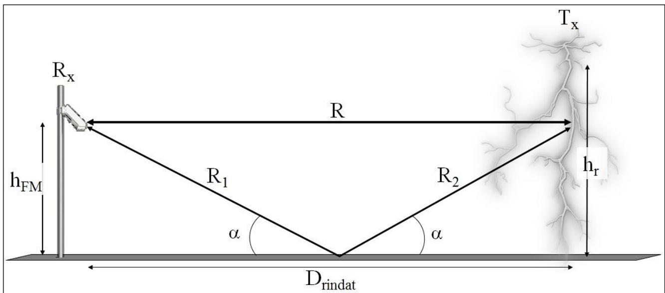
**Figure 1.** Concept of a transmitting (lightning -  $T_x$ ) and receiving (Field Mill -  $R_x$ ) antenna, where  $R$  is the distance between  $T_x$  and  $R_x$ ,  $D_{rindat}$  is the distance [m], predicted by the lightning discharge detection system (RINDAT). Source: The authors (2022).
