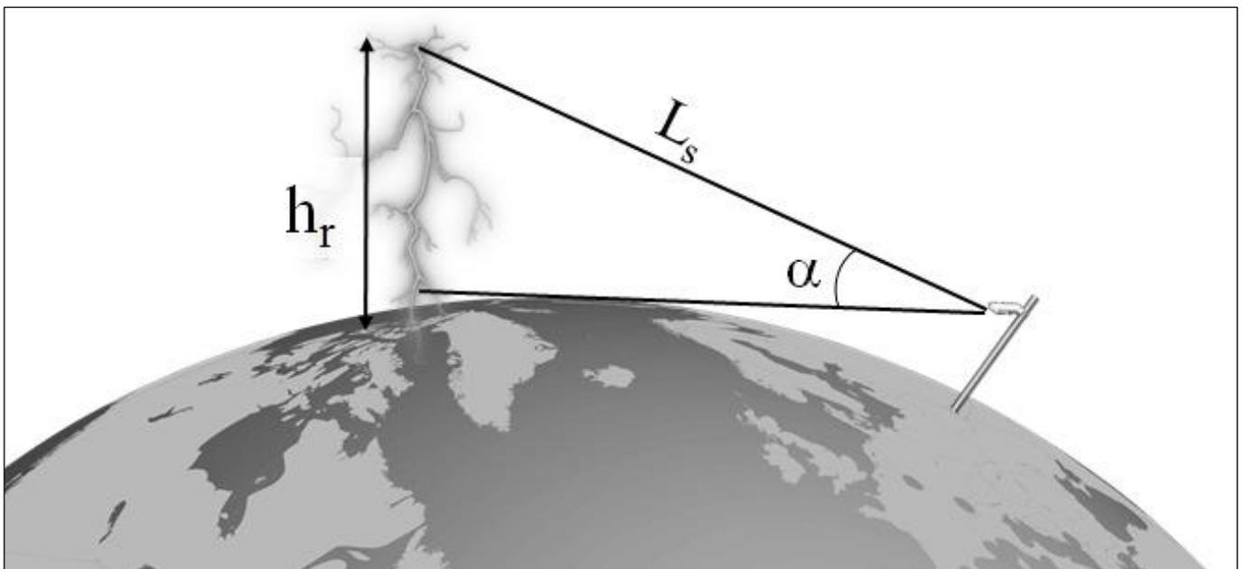
**Figure 2.** Model of a satellite radio link adapted to the case of an atmospheric electric field sensor and a lightning discharge. Graphic representation is not to scale. Source: The authors (2022).
