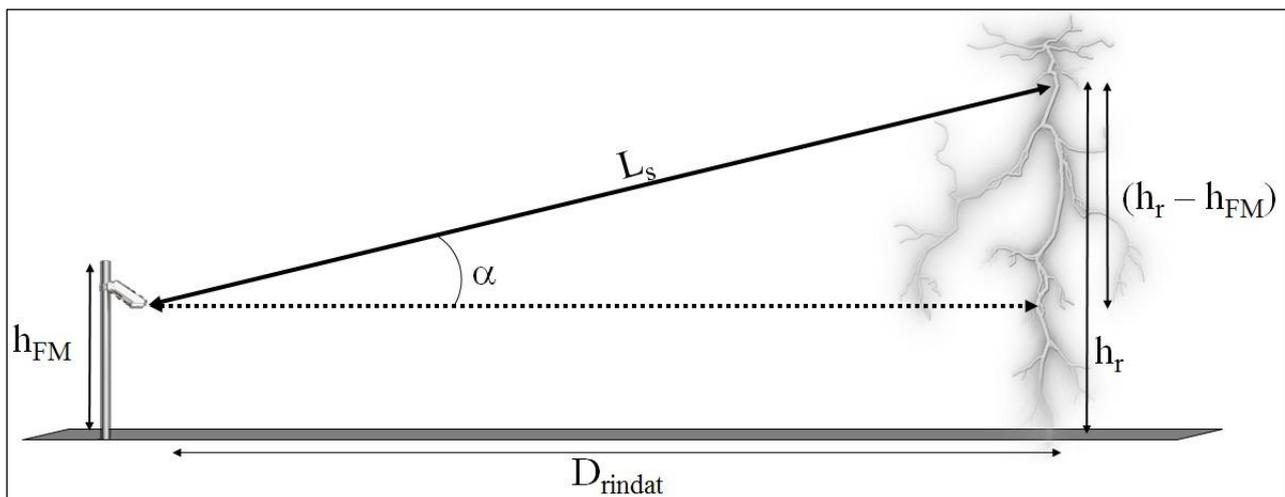
**Figure 3.** Relation between the system's heights  $R_x$  (Field Mill) and  $T_x$  (lightning) and minimum elevation angle.
