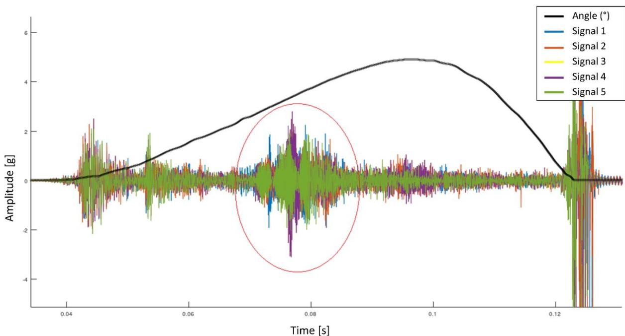
**Figure 6.** HVCB vibration signals in fault 1 condition.
