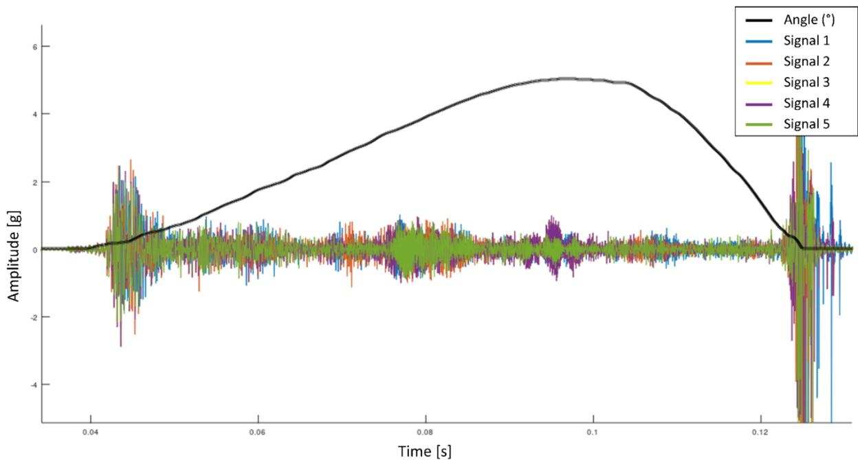
**Figure 5.** HVCB vibration signals in healthy condition.
