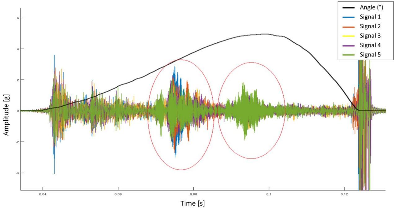
**Figure 7.** HVCB vibration signals in fault 2 condition.
