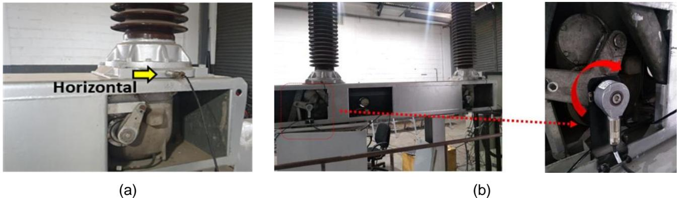
**Figure 2. (a):** installed accelerometer position. **(b):** installed incremental encoders position.
