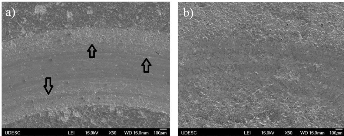
Figure 9: SEM micrographs of wear tracks a) Q/T-TiN b) B-TiN.
