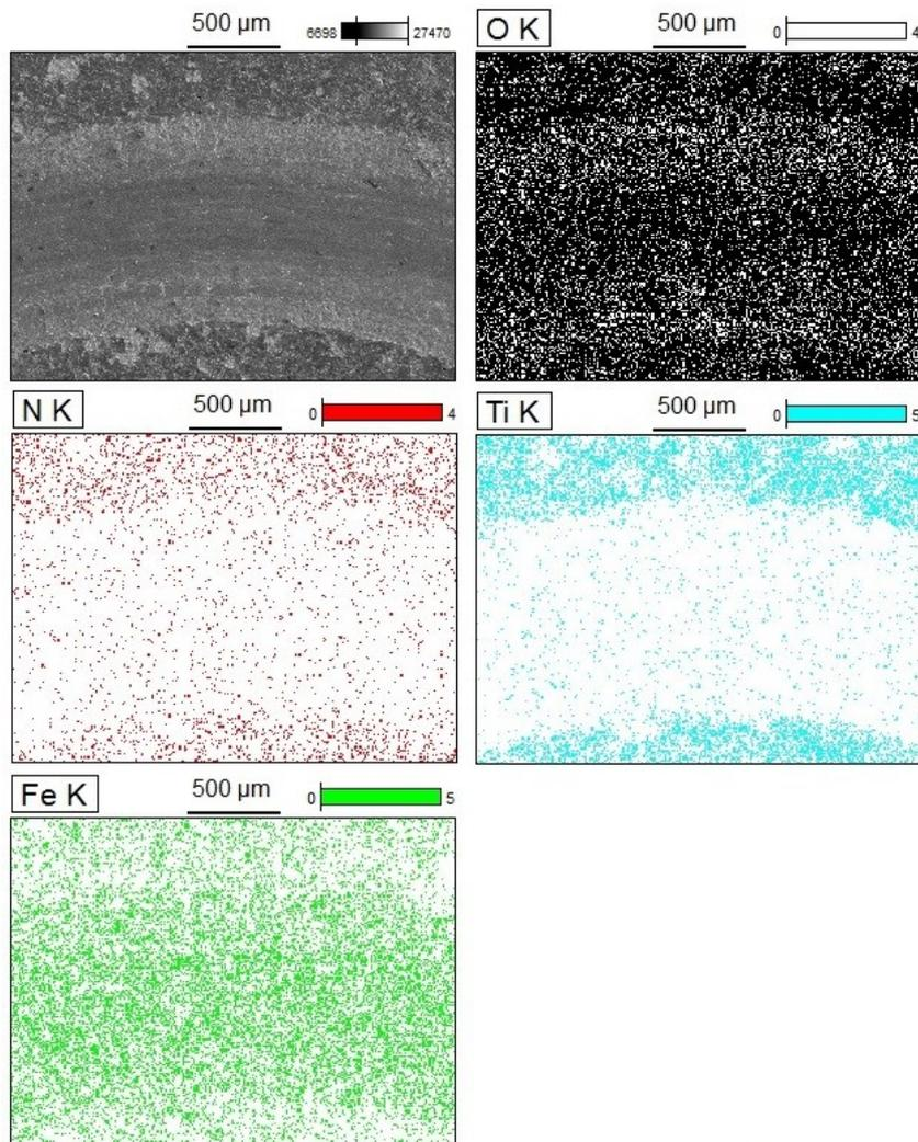
Figure 10: Worn track and EDS mapping of Q/T-TiN sample.
