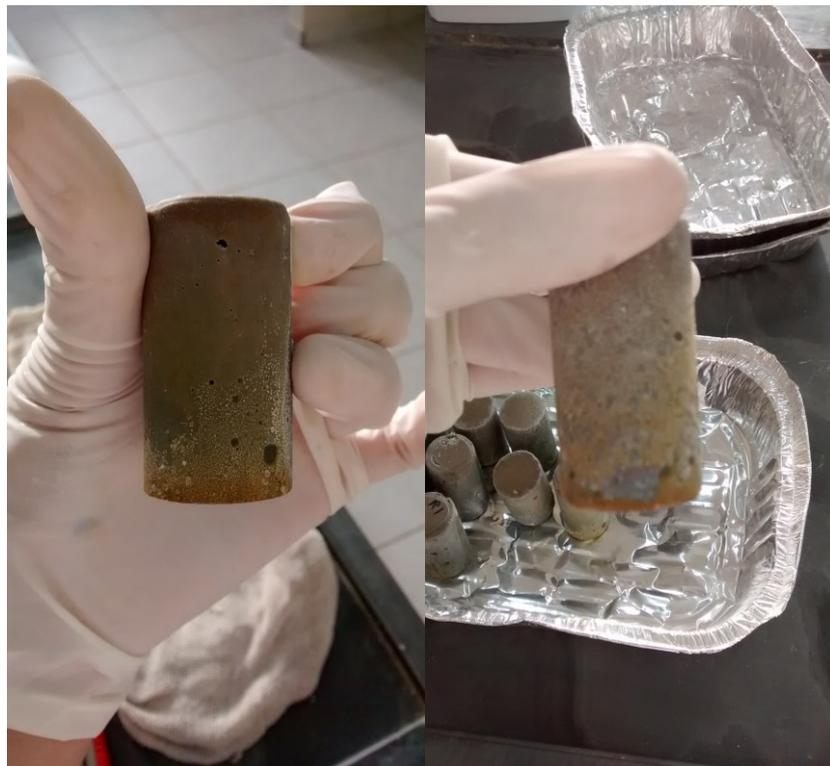
**Figure 11:** Samples after chemical attack.
