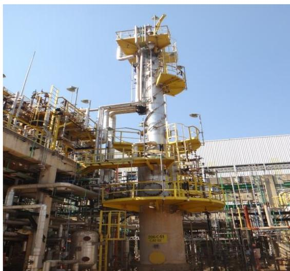
**Figure 3:** The DEA regenerating tower in the oil refinery.
