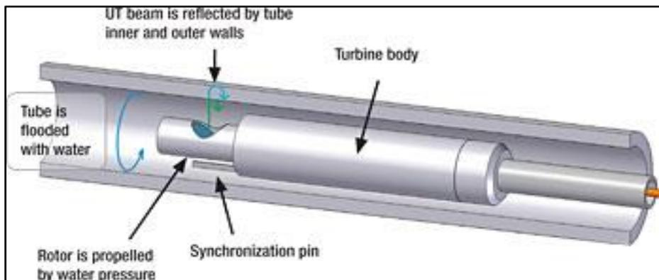
**Figure 6:** Probe turbine assembly.
