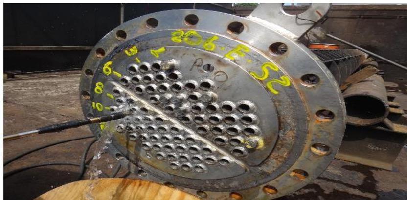
**Figure 5:** Internal Rotation Inspection (IRIS) equipment test.
