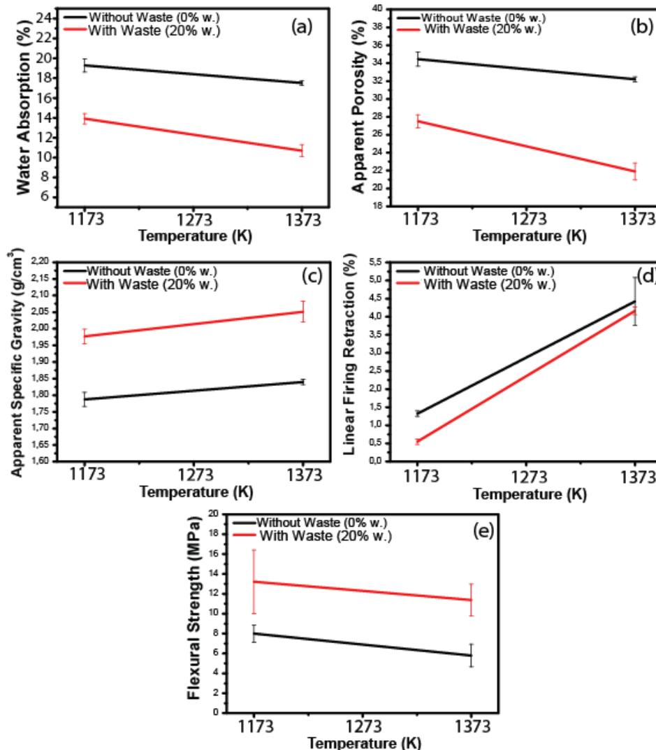
**Figure 4:** (a) Water absorption; (b) apparent porosity; (c) apparent specific mass; (d) linear firing retraction; (e) flexural strength module.
