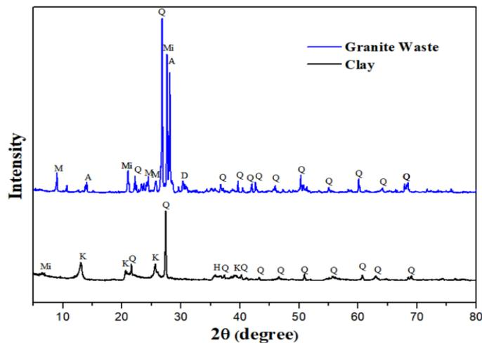
**Figure 1:** X-ray diffractogram of the granite waste; and diffractogram of the clay: Q - quartz, M - muscovite, Mi - microcline, D - dolomite, A - albite, H - hematite and K - kaolinite.
