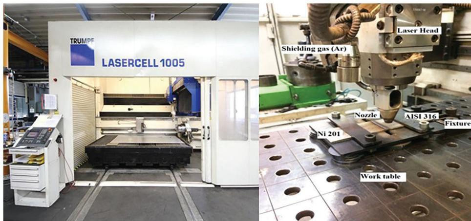
**Figure 1:** Experimental setup of TRUMPF LASERCELL TLC1005.
