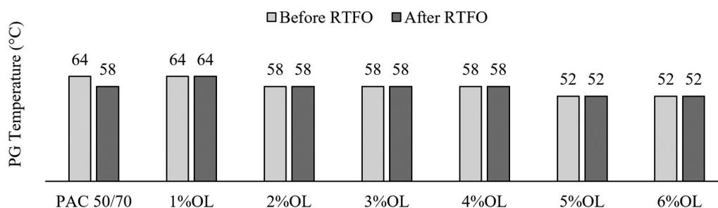
Figure 1: Performance grading of asphalt binders.
