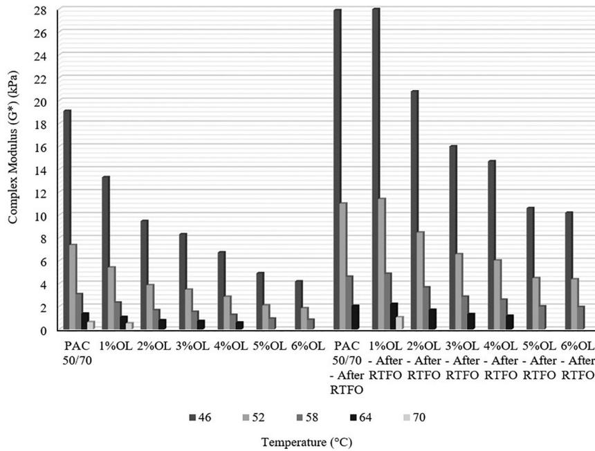
Figure 2: Complex Modulus Parameter ( $G^*$ ) as a function of temperature before and after RTFO.
