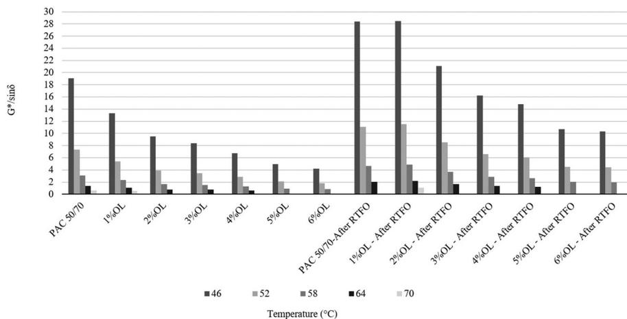
Figure 3: Parameter  $G^*/\sin\delta$  as a function of temperature before and after RTFO.
