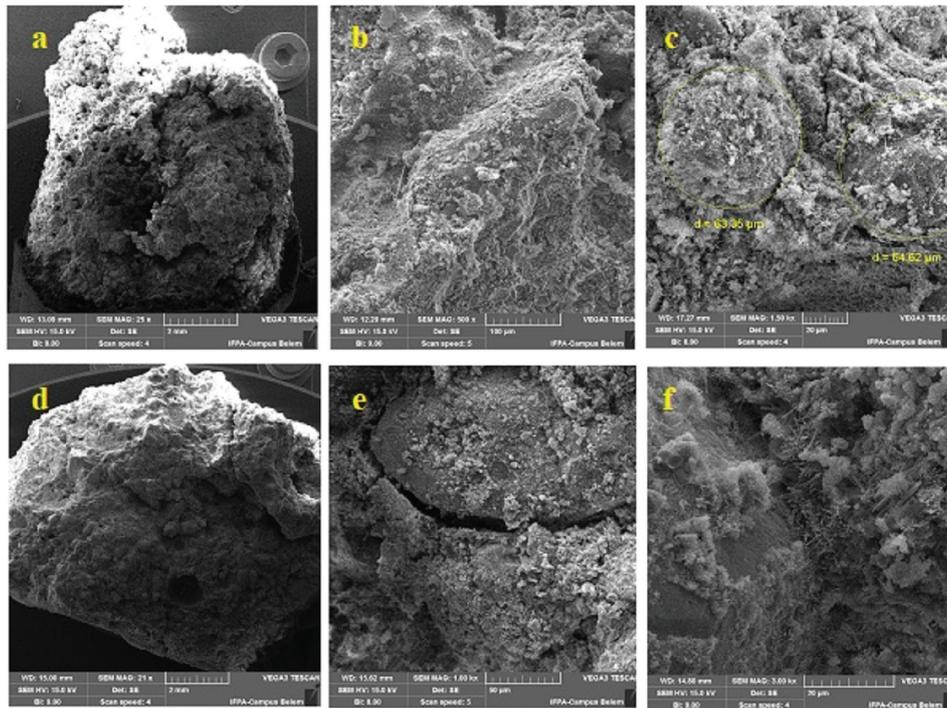
**Figure 7:** Microstructure SEM images of the mortar samples breakage of the Axial Compressive Strength: a) RQA fragments; b) RQA mortar sample with adherence; c) breakage sample of mortar sample with cement crystals; d) Reference fragments; e) CRE mortar sample with adherence; f) breakage of CRE mortar sample.
