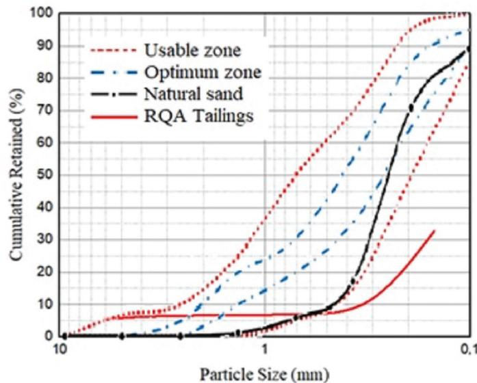
Figure 5: Particle size distribution of natural sand and RQA tailings aggregates.
