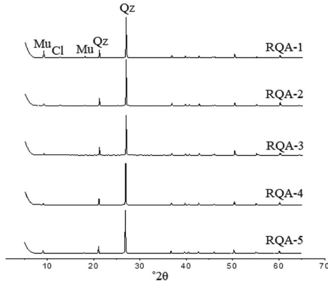
Figure 4: Diffractograms of amethyst quartz tailings.
