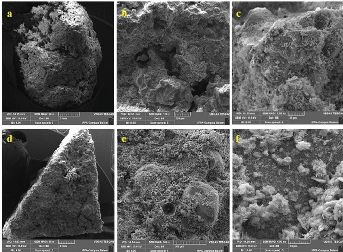
**Figure 8:** Microstructure SEM images of the mortar samples breakage of the Flexural Tensile Strength: a) RQA fragments; b) RQA mortar sample with adherence; c) breakage sample of mortar sample with cement crystals; d) Reference fragments; e) CRE mortar sample with adherence; f) breakage sample of CRE mortar sample.
