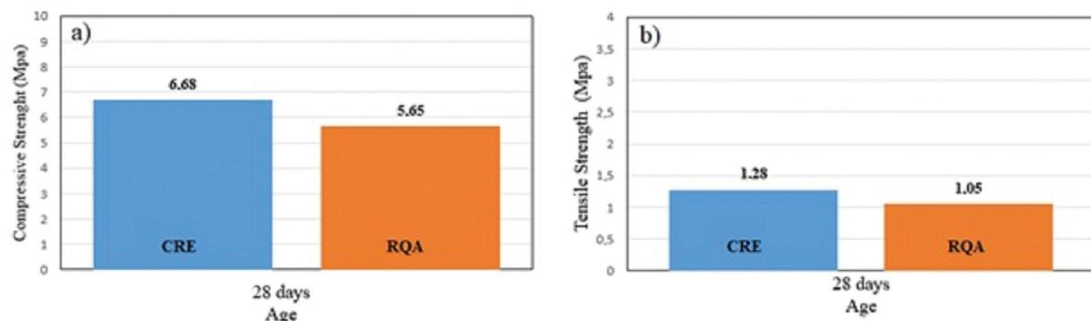
**Figure 6:** a) Axial compressive strength of natural sand CRE and tailings RQA mortars b) Flexural tensile strength of the natural sand CRE and tailings RQA mortars. Trace 1:3.
