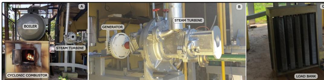
**Figure 2:** The experimental bench used in the study, cyclonic combustion boiler and steam turbine (A), permanent magnet electric generator and steam turbine (B) and resistive load bank (C).
