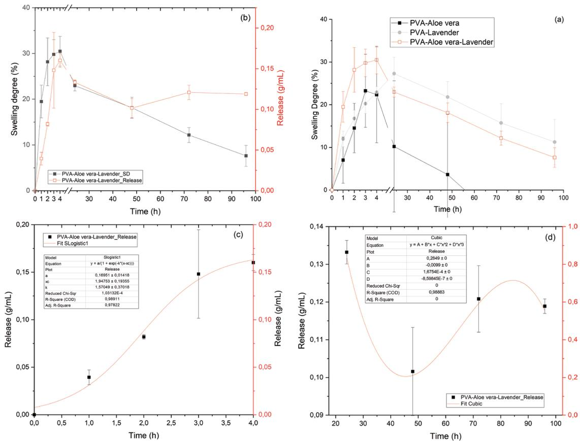
**Figure 7:** PVA-Aloe vera-Lavender essential oil (a) swelling degree, (b) swelling degree compared to the release of the combined actives; (c) initial release modeled; (d) long-term release modeled.
