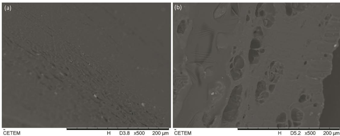
**Figure 4:** SEM analysis of (a) PVA hydrogel and (b) PVA-Lavender hydrogel.
