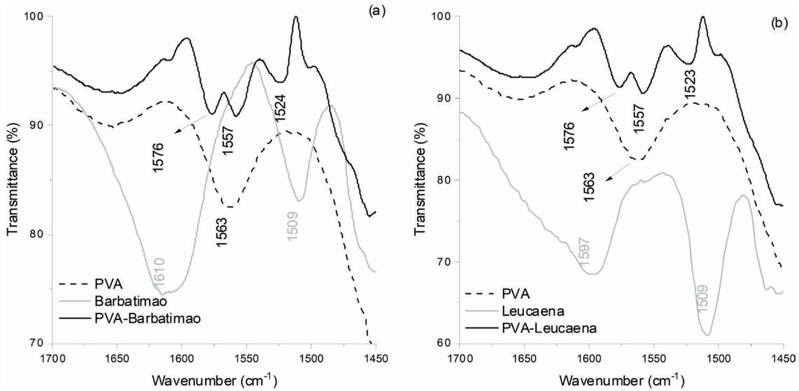
**Figure 3:** FTIR spectra of the raw materials, as well as (a) PVA-Barbatimão and (b) PVA-Leucaena, in the region of wavenumbers between 1700 and 1450  $\text{cm}^{-1}$ .
