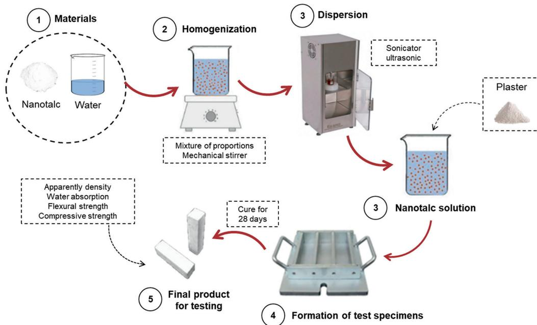
**Figure 1:** Representative scheme of the production of nanocomposite test specimens.
