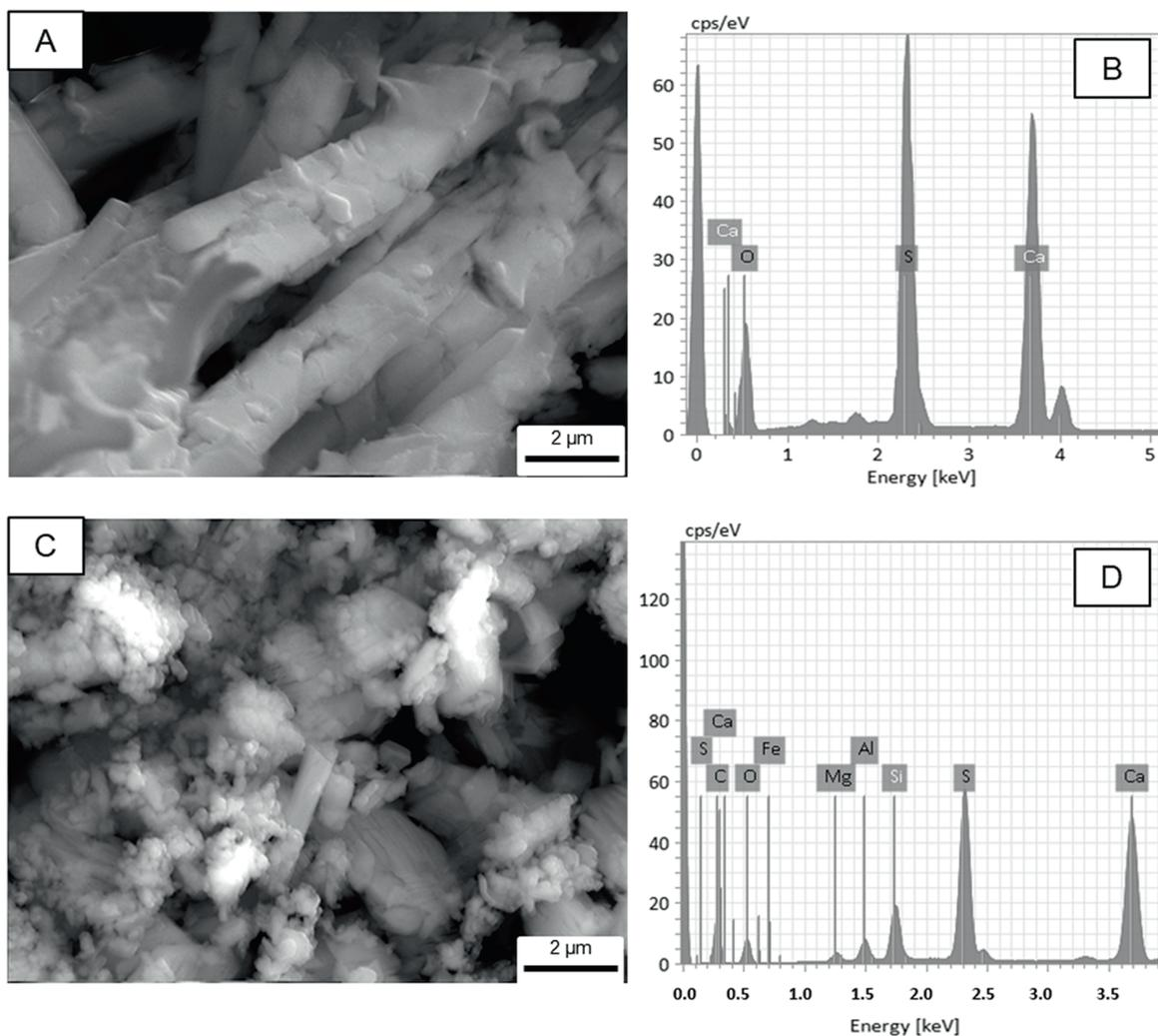
**Figure 6:** Scanning electron micrograph and EDS of the samples, being (a,b) without addition of nanotalc and (b,d) 1% of nanotalc.
