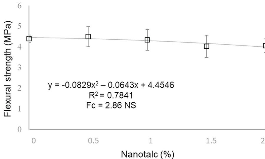
**Figure 4:** Flexural rupture modulus of the produced nanocomposites.
