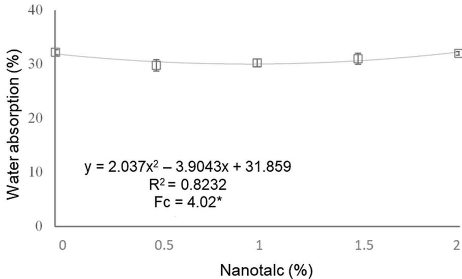
**Figure 3:** Water absorption of the produced nanocomposites.
