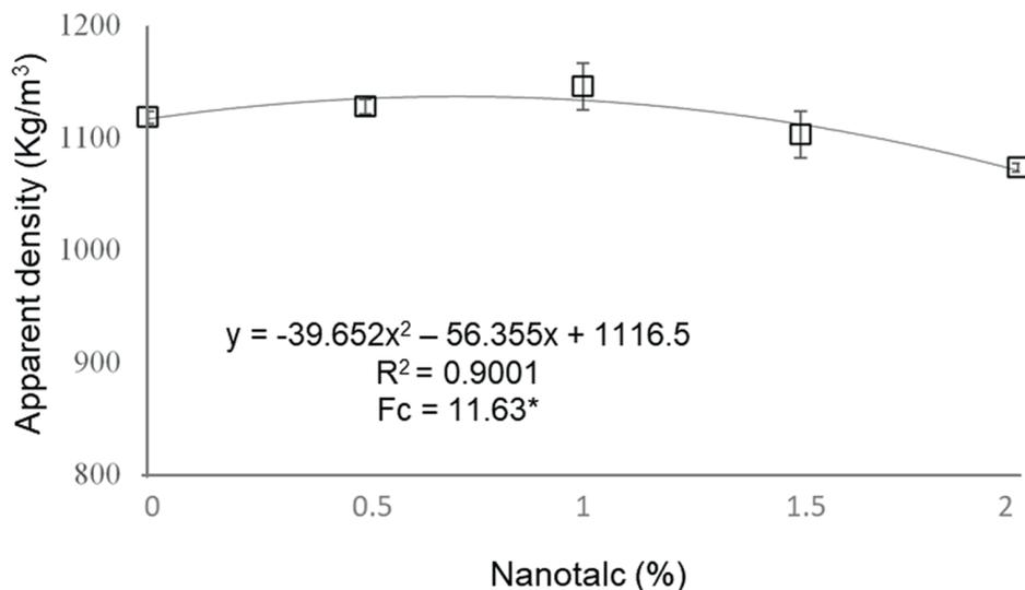
**Figure 2:** Apparent density of the produced nanocomposites.
