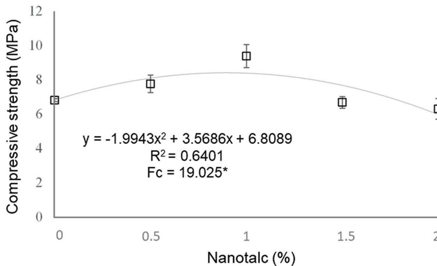
**Figure 5:** Compressive strength of the produced nanocomposites.
