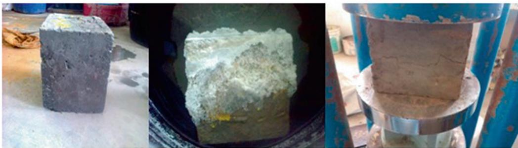
**Figure 7:** Typical surface profile and failure pattern of cube after sulphate attack.
