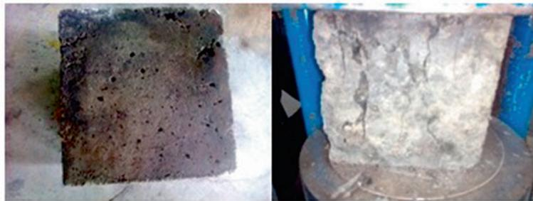
**Figure 8:** Typical surface profile and failure pattern of cube after chloride attack.
