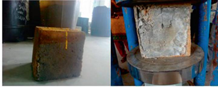
**Figure 6:** Typical surface profile and failure pattern of cube after acid attack.
