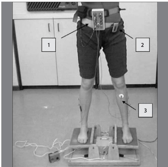
**Figure 1.** Athletes position on the electronic platform: (1) = EMG patients unit; (2) = Radio-phon gear; (3) = Ground electrode.
