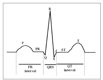
Figure 2. ECG signal waveform.
