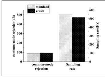
Figure 8. Common mode rejection and sampling rate test results.
