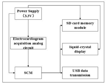
Figure 3. ECG data acquisition board.
