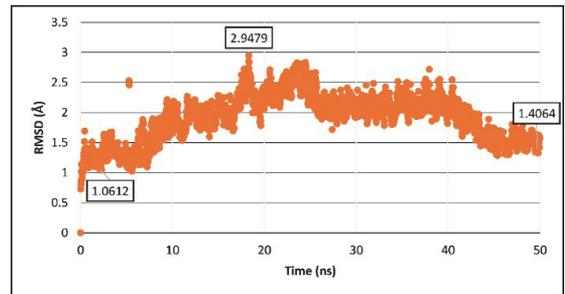
**Figure 1.** RMSD of TQ and Mpro during the 50ns MD simulation period. Stability seems fluctuating from 1.0612Å at 2ns and 2.94 Å at 18ns. Target stability seems unstable even at the end of simulation period.
