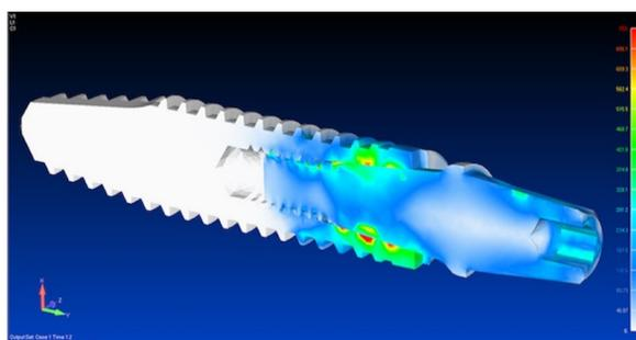
**Figure 8.** Finite element analysis of the CM group: stress accumulation is represented in the red color located in the region with no contact of abutment/implant.
