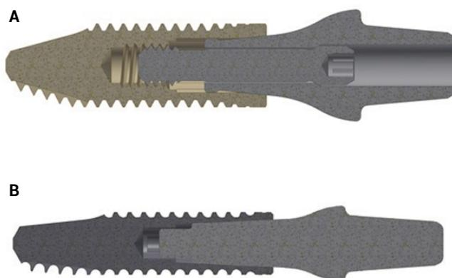
**Figure 1.** A) CM implants - Morse taper implants with 11.5° angulation of the internal conical portion and 3.5mm in diameter. B) FAC group implants (FAC) - Morse taper self-locking implants with 5° angulation of the internal conical portion and 2.9 mm in diameter.
