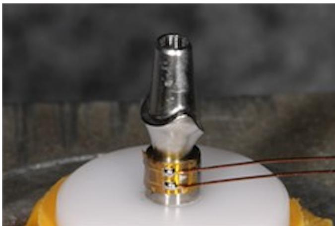
**Figure 3.** Strain gauge fixed in the cervical portion of the implant. Note that the implant was fabricated without external threads to permit this fixation.
