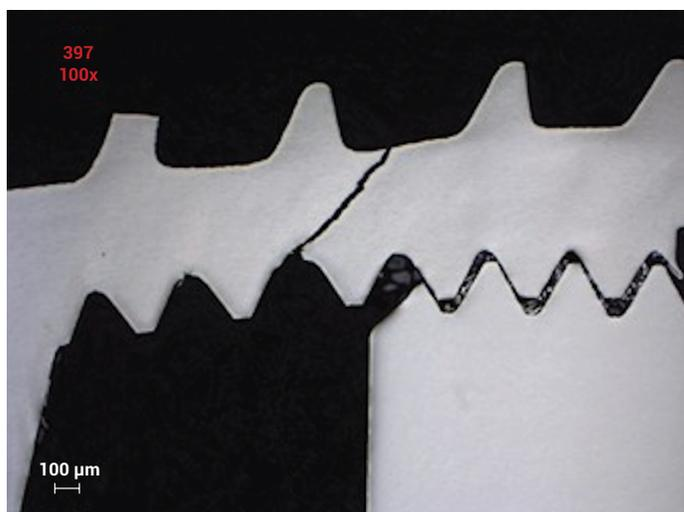
**Figure 5.** Optical microscopic evaluation: implant fracture at the discontinuity region of the abutment/implant interface (approximated view). - CM group.
