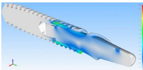
**Figure 7.** Finite element analysis of the FAC group implants: stress accumulation is represented in the red color located in the region with no contact of abutment/implant.
