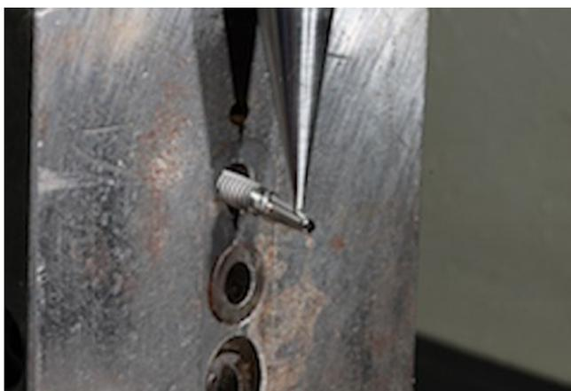
**Figure 2.** The implant and the metallic holder were fixed on the mechanical testing machine (EMIC; 2000DL) and submitted to a load cell of 500 KN capacity (KN500; EMIC).
