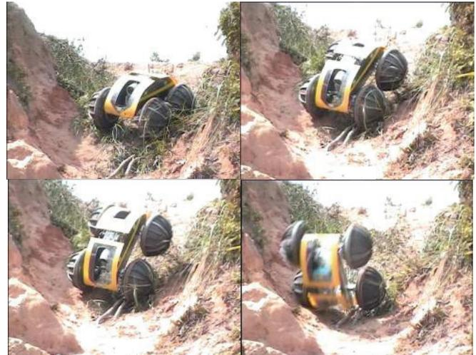
Figure 9. Rough terrain experiment with the first prototype of the Hybrid Environmental Robot without traction control, showing flip-over instability.
