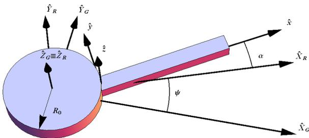
Figure 1. Reference frames of the rotating beam.
