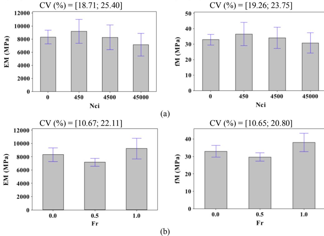
Table 4 presents the results of the Tukey test of mechanical properties as a function of the two factors evaluated (Nci and Fr) for Cambará. The multivariable regression models and the respective determination coefficients for the estimation of the values of the modulus of elasticity and of the rupture module in static bending for Cambará wood are expressed by Equations 9 and 10, respectively. The model was significant by the ANOVA, with p-value below 5%.
