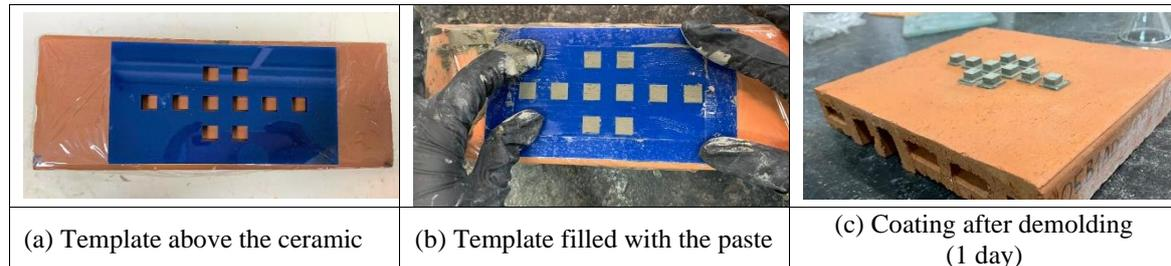
Figure 3 - Methodology for testing tensile bond strength
