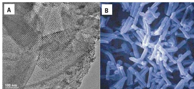
**Figure 1.** Mesoporous nanostructured SBA-15. (A) Transmission Electron Microscopy (TEM) of SBA-15 silica, highlighting its hexagonal ordered porous structure with mean pore diameter of around 10 nm. (B) Scanning Electron Microscopy (SEM) picture of SBA-15 particles of around 30  $\mu\text{m}$  in diameter, showing their macroporous morphology
