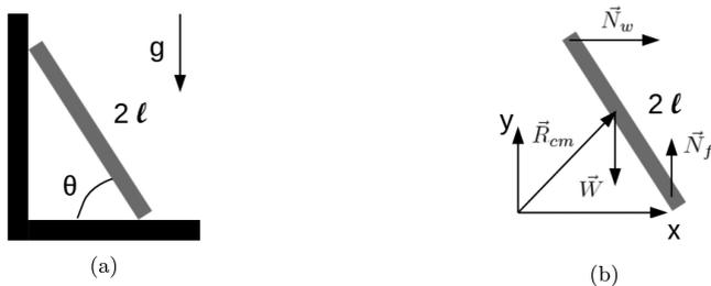
**Figure 2:** (a) A ladder of length  $2\ell$  starts to slide from rest on a frictionless surface and (b) forces acting on the ladder.
