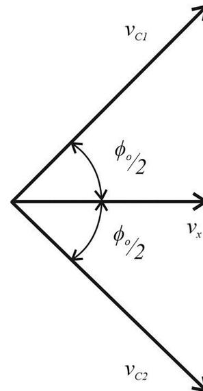
**Figure 6:** Representation of  $v_{C1}$ ,  $v_{C2}$  and  $v_x$  at the instant  $t = 0$ .
