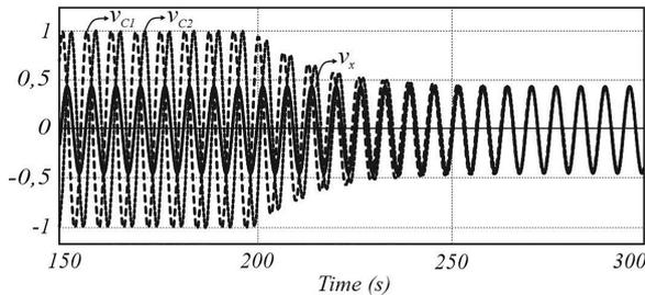
**Figure 5:** Voltages  $v_{C1}$ ,  $v_{C2}$  and  $v_x$  as a function of time, during the phase synchronization transient.
