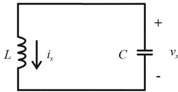
**Figure 4:** Equivalent circuit described by the second order differential equation (35).
