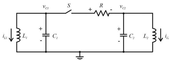
Figure 1: Two coupled identical linear LC oscillators.
