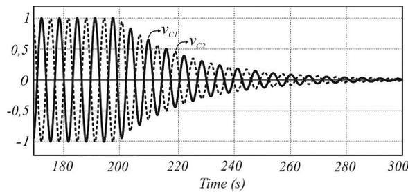
**Figure 10:** Representation of voltages  $v_{C1}$  and  $v_{C2}$  across the capacitors for  $\phi_o = \pi$ , with  $R = 20\Omega$ ,  $C = 1F$ ,  $L = 1H$  and  $V_p = 1V$ .
