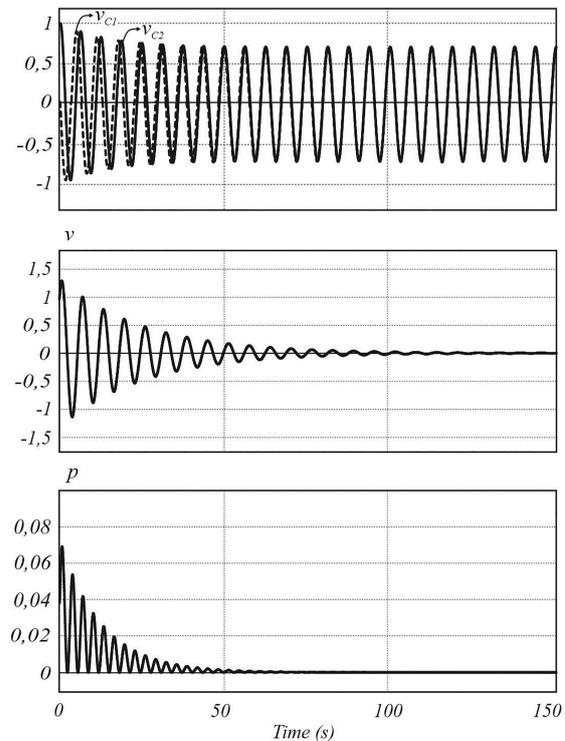
**Figure 3:** Typical waveforms for the voltages  $v_{C1}$  and  $v_{C2}$  across the capacitors, the voltage  $v$  across the coupling resistor  $R$  and the instantaneous power  $p$  dissipated in  $R$ .
