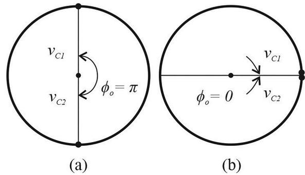
**Figure 11:** Representation of initial phase between voltages  $v_{C1}$  and  $v_{C2}$ . (a)  $\phi_o = \pi$  and (b)  $\phi_o = 0$ .
