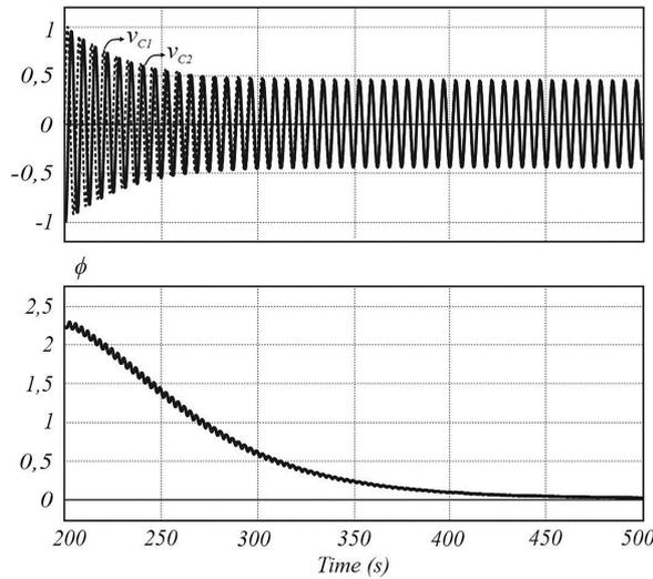
**Figure 9:** Representation of voltages  $v_{C1}$  and  $v_{C2}$  across the capacitors and  $\phi$  for  $\phi_o = 2.23rd$ , with  $R = 50\Omega$ ,  $C = 1F$ ,  $L = 1H$  and  $V_p = 1V$ .
