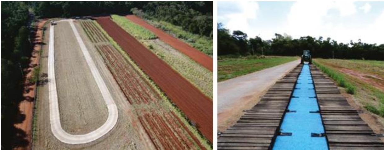
Figure 7 - Standardized tracks for agricultural tractor testing, from left to right: OECD oval concrete track; mobilized soil track; conventional soil-in-preparation track; no-tillage soil track, firm soil track, and ISO 5008 tractor vibration track
