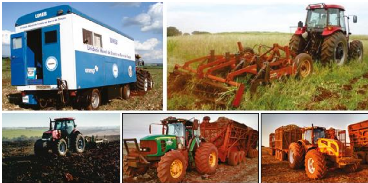
Figure 4 - Field tests to assess tractor performance with a dynamometer car; subsoiler; tipping trailer. NEMPA/Botucatu 2018
