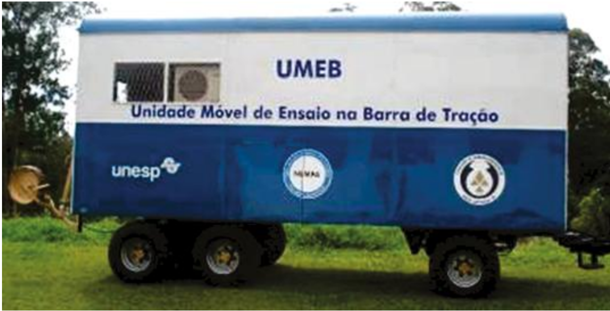
Figure 2 - Dynamometer unit for the application of controlled loads in drawbar performance tests. NEMPA/Botucatu 2018
