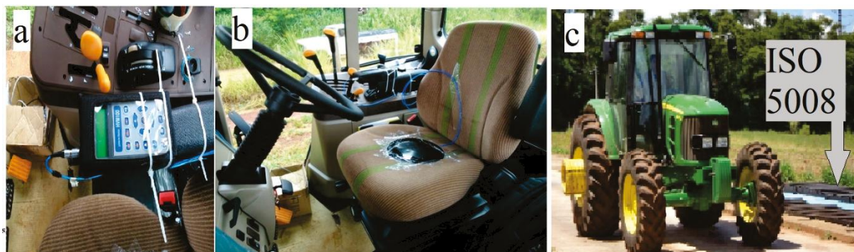
Figure 5 - Vibration tests on a standardized surface: a. datalogger system; b. vibration sensor in the operator seat; c. instrumented tractor on an ISO 5008 standardized surface
