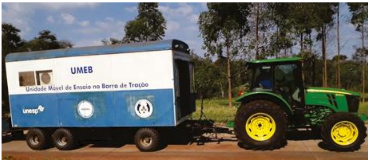
Figure 9 - Drawbar test mobile unit - UMEB
