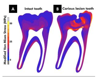
**Figure 3.** Mvm stress distribution for no restored finite element models of molar teeth during 100 N functional bite loading: A. Intact tooth; B. Dcl, with deep carious lesion.
