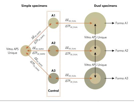
Figure 1. A schematic showing the specimen arrangement used to calculate color differences.
