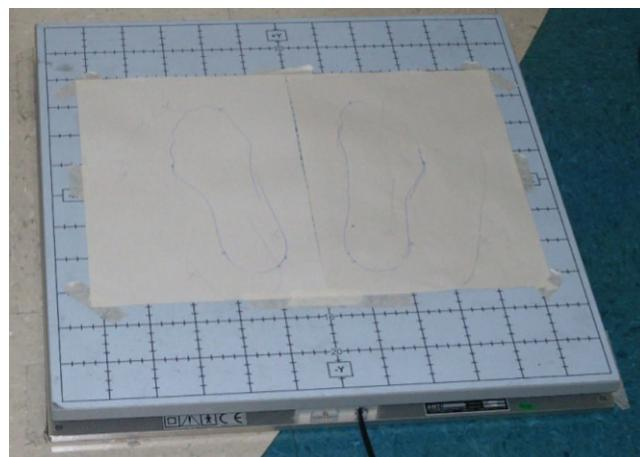
Figure 1 - AccuSway<sup>Plus</sup> portable force platform.
