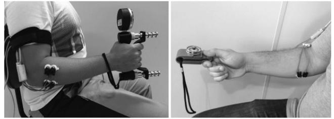
Figure 2: Positioning of electrodes for EMG signal capture of extensor carpi ulnaris (ECU), extensor carpi radialis (ECR) and flexor digitorum superficialis (FDS) muscles during the task of palmar grip strength and lateral pinch.
