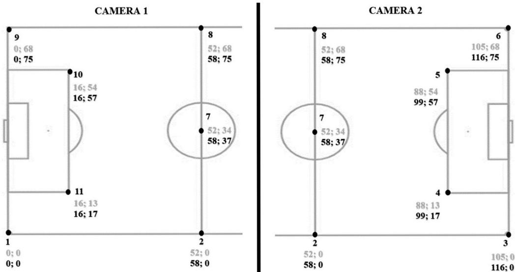
**Figure 1** - Calibration points (1 to 11) for each half of the pitch and the respective position for a field measuring 105 m x 68 m (grey) and 116 m x 75 m (black).
