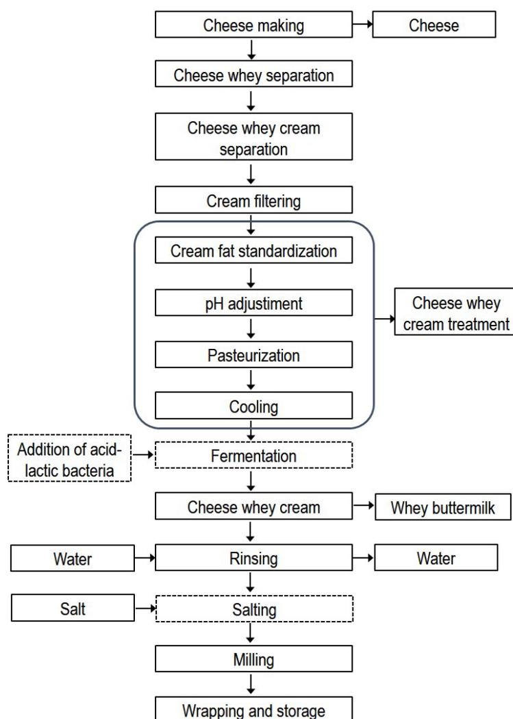
**Figure 2.** Flowchart of the whey cream butter-making process.
