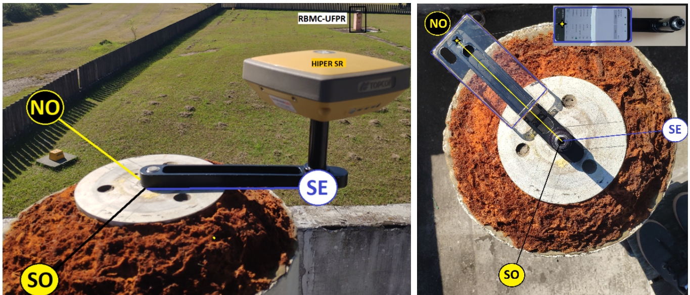
Figure 1: On the left, the figure shows the geodetic receiver HiPer SR positioned above the rod in the SE auxiliary position. In the background, the RBMC-UFPR station. On the right, the figure shows the position of Mi 8 in relation to the rod and above the NO auxiliary point.
