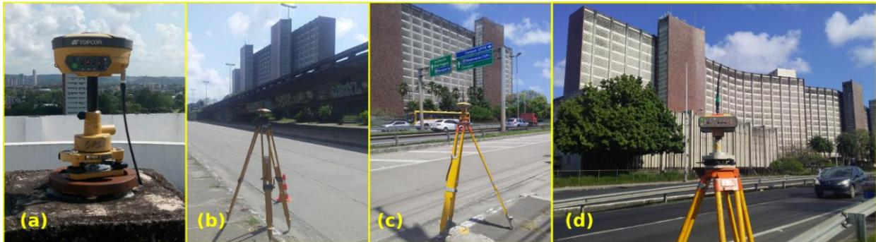
**Figure 2:** (a) GNSS Topcon Hiper V receiver at SAT GPS station 91551; (b), (c) and (d) GNSS Topcon Hiper Lite<sup>+</sup> receivers measuring the immediate support points (P1, P2 and P3 respectively) near the building.
