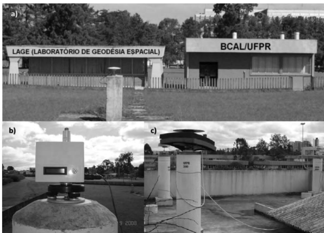
**Figure S1:** a) BCAL/UFPR Calibration Basis; b) DRB calibration device; c) Calibration pillars.
