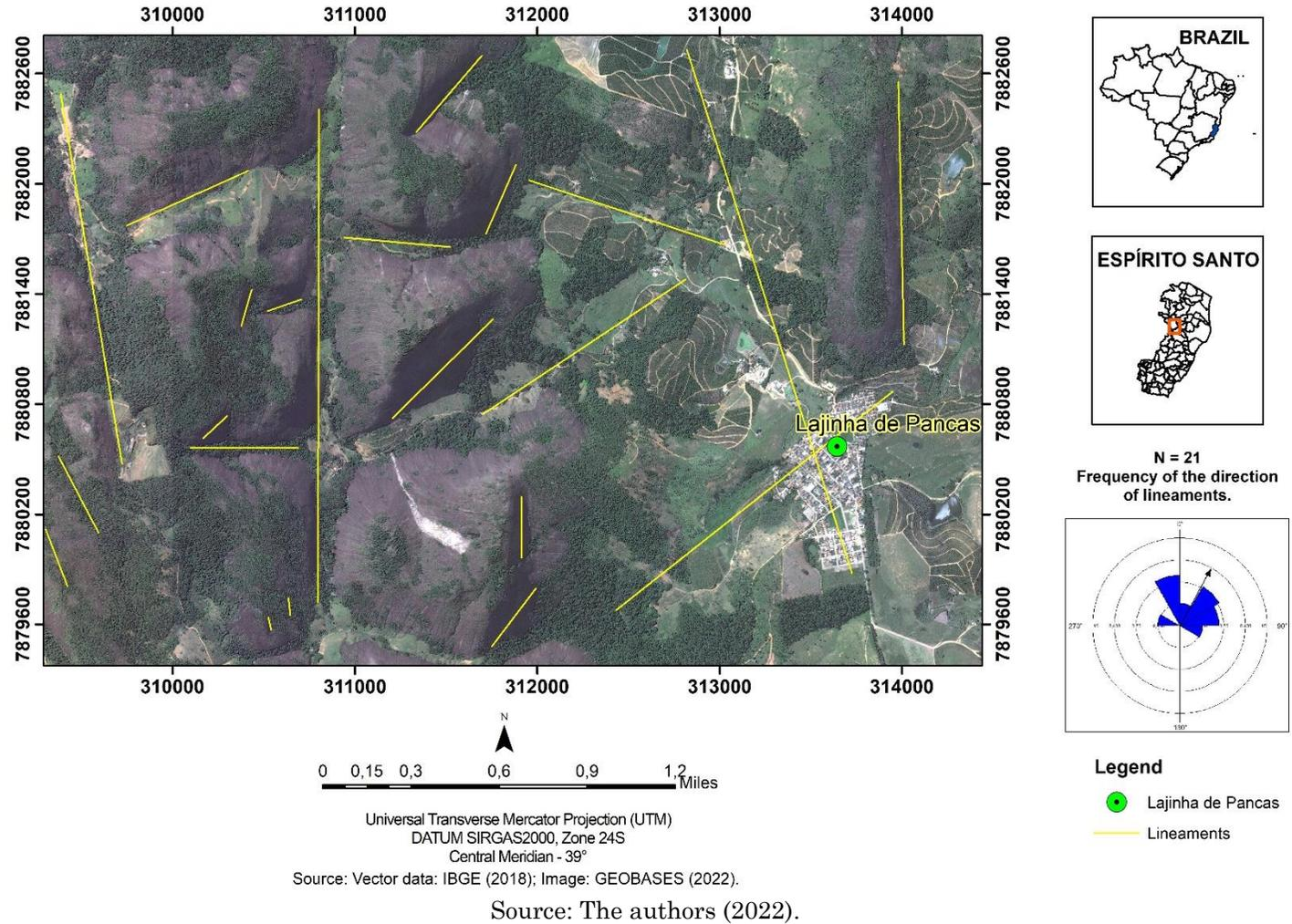
The rosette chart of the existing fault and fracture map in the studied area showed the predominance of lineaments in the NNW-SSE and NW-SE directions, followed by the NNE-SSW and NE-SW and the WNW-ESE and ENE-
