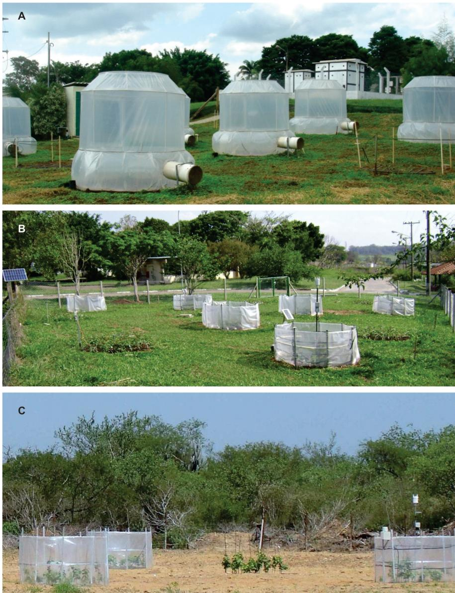
**FIGURE 4** - Open-top chambers for studying the impacts of increased air CO<sub>2</sub> concentration (A-B. Jaguariúna SP, Brazil; and C. in Petrolina, PE, Brazil).
