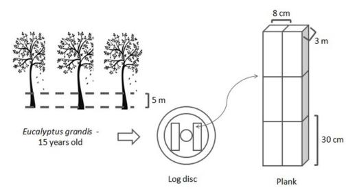
Figure 1. Schematics of the material obtainment: selection of three trees, demarcation of the heart region, plank extraction and test specimen production with dimensions of  $30 \times 8 \times 3$  cm (length × width × thickness, respectively).
