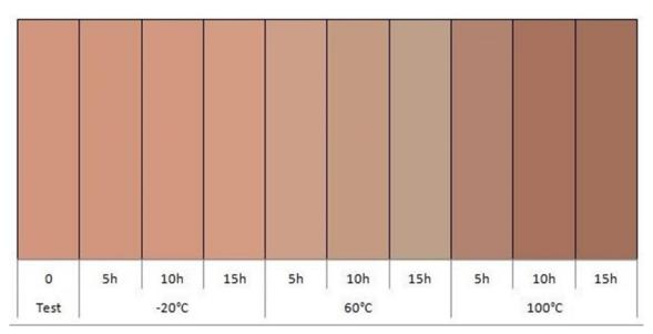
**Figure 3**. Representation of *Eucalyptus grandis* wood submitted to thermal treatment (temperatures: -20, 60, and 100°C and exposure time: 5, 10, and 15 h), and also the *in natura* wood (control).
