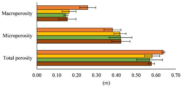
Figure 3. Macro, micro, and total porosity ( $m^3 m^{-3}$ ) of the experimental area in the treatments: previous (before silage harvest), T1, T2, and T2 with transport wagon in the layer of 0.2 - 0.4 m.
