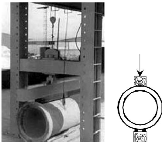
The ultimate (collapse) load is the maximum force achieved in the diametral compression test, which leads to the ultimate limit state for the pipe. The service load is one for which a crack with opening of 0,25 mm will appear in the pipe, with a length of 300 mm or more, which corresponds to the service (cracking) limit state.
