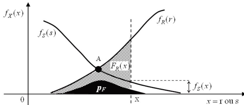
probability is evaluated by Equation 7, where  $f_X(x)$  is the joint probability density function and  $D_f$  is the failure domain, defined by limit state equation  $g(\mathbf{X})$ , written in function of design variables  $\mathbf{X}$ .
