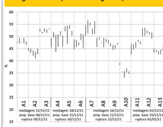
Figure 2 – Profile of variations in compressive strength, consistency and coarse aggregate content – lots 1 to 4
