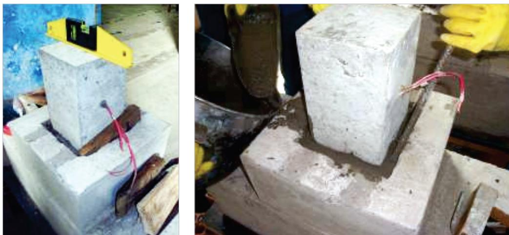
Figure 7 illustrates the positioning of the column and the filling of the grout.
