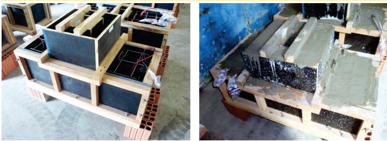
Figure 7 – Positioning of column in socket foundation and grout filling
