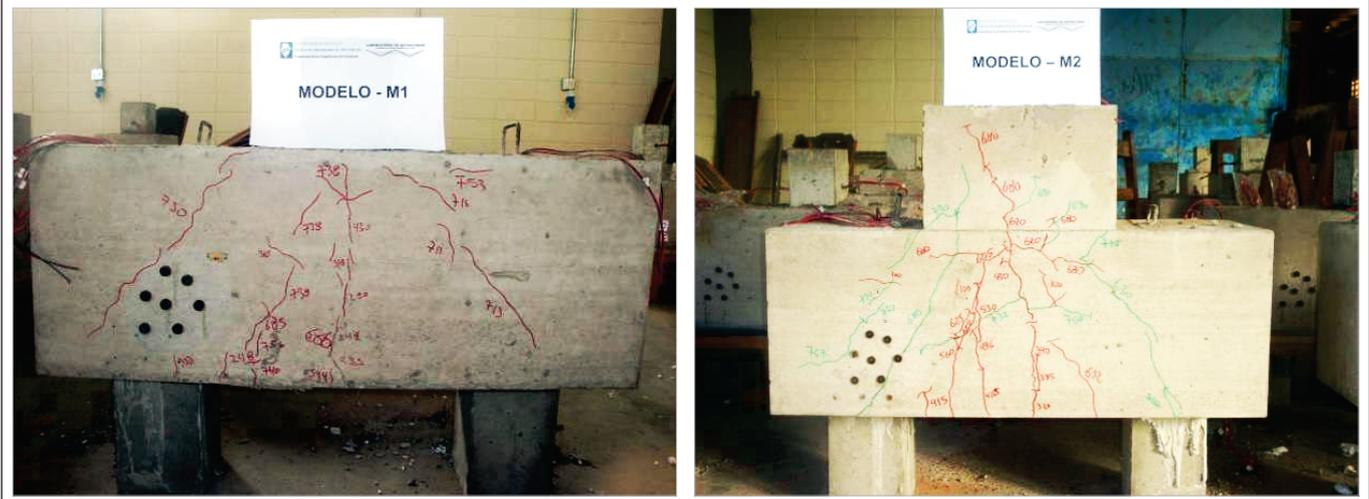
ued until the upper region. It was also observed the formation of horizontal cracks in the region of the socket at loads near the ruin of the model. Figure 11 shows the overview cracking from M1 and M2 models.
