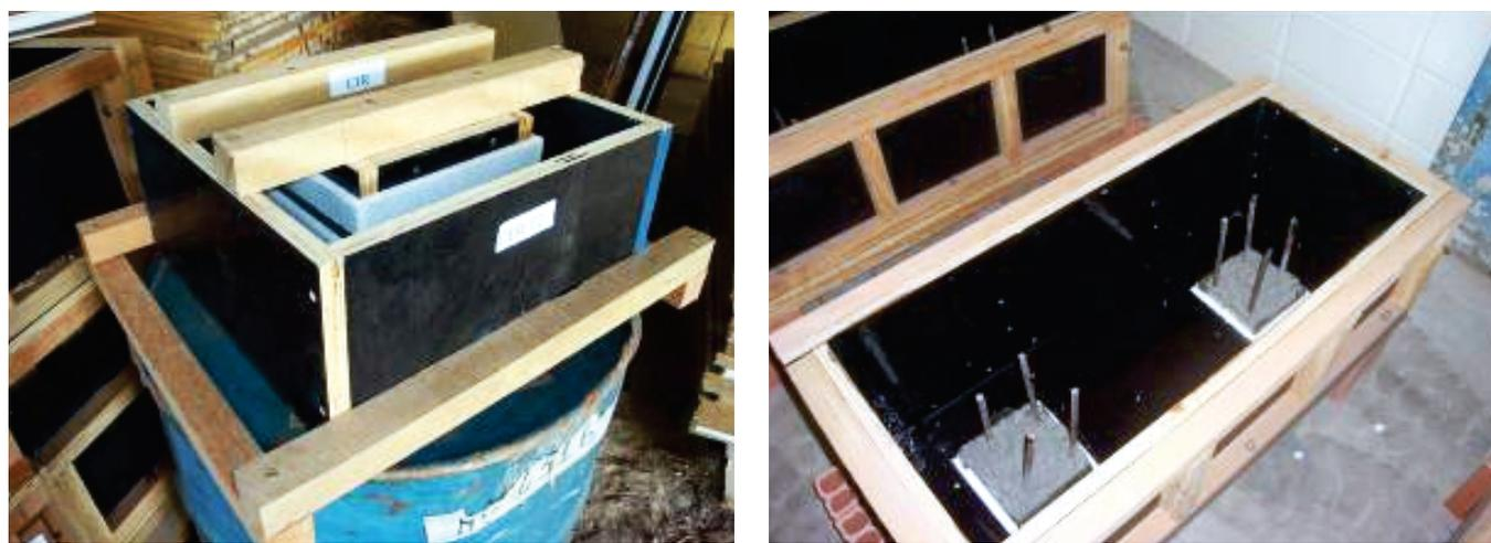
in their bars. Then the reinforcement bars of the columns were assembled, and finally, the reinforcement bars of pile caps along with the sockets. Figure 4 shows the stage of design and the reinforcement bars of the columns after assembly, and figure 5 shows the assembly of the reinforcement bars of the pile cap.
