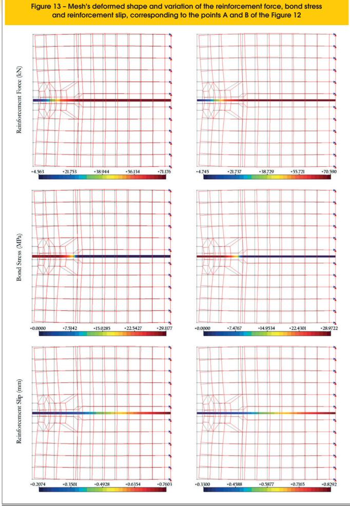
In order to explain this occurrence, Figure 13 shows the variation of the reinforcement force, bond stress and reinforcement slip, as well as the mesh's deformed shape, corresponding to the points A (right images) and B (left images) of the Figure 12.
