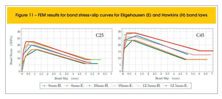
Nonlinear simulations have been performed under the assumption of plane stress conditions and using generalized displacement control method (Yang and Shieh [28]), initial load factor equal to  $0.080\,$  and  $0.040\,$  for Eligehausen [18] and Hawkins [19] bond laws, respectively, and tolerance of  $1\times10^{-4}\,$ .
