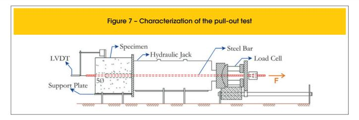
specimen. This test has aimed to study the relationship between bond stress and bond loss of the steel bar. Both ends of the bar are designed for out of the specimen, so that, the pull-out force is applied at one end while the bond loss is measured at the opposite end (Figure 7).
